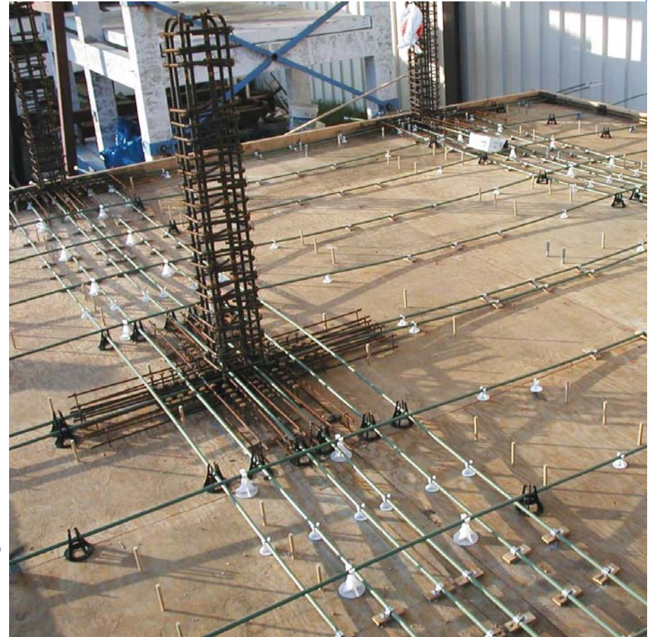
\sim 1/3 scale shake table test specimen
