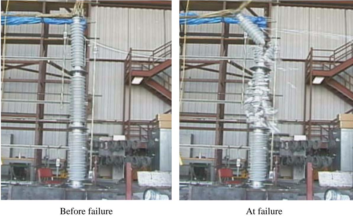
Fig. 3- Static cantilever strength testing of the porcelain insulator posts
