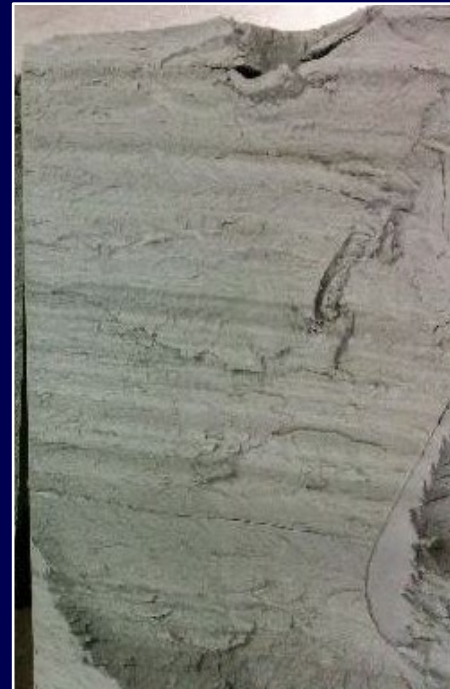
PI = 10 Silt (S33-DM1-8U-A)
