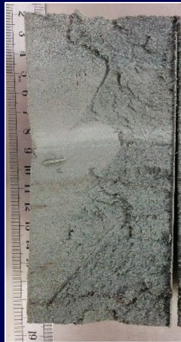
PI = 0 Silt (S33-DM1-6U-B)
