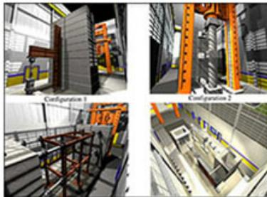
The single degree of freedom shaking table has a maximum stroke of +/-20 in. The platform is 7 ft × 19 ft. The payload can be as high as 200 kips, with lateral capacity of 150 kips. The controller is connected to a SCRAMNet ring buffer; hence, this shaking table is capable of performing real-time hybrid simulation. This platform is ideal for projects requiring large displacement such as seismically isolated structures or large velocity such as the floor response of multi-story buildings.
