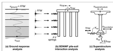
The impact of this research will be the improved assessment of the seismic response of bridges founded on deep foundations, particularly for large-diameter stiff foundations in soft soils. Piles that are restrained rotationally by a pile cap result in the foundation input motion being lower than the free-field motion, particularly at high frequencies. Free-head piles exhibit
