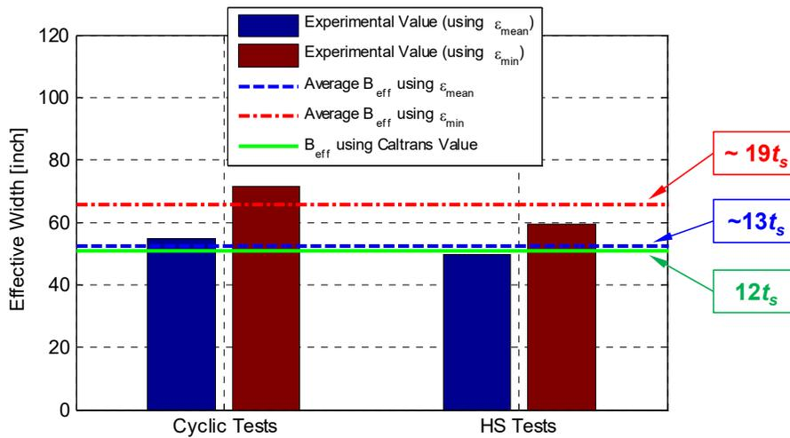
**Figure 3.89** Average values for the effective flange width to be added to the cap beam width from the as-built Specimen No. 1 cyclic tests and the retrofitted Specimen No. 2 HS tests and overall mean value from all tests when the cap beam minimum and mean strain values were used.
