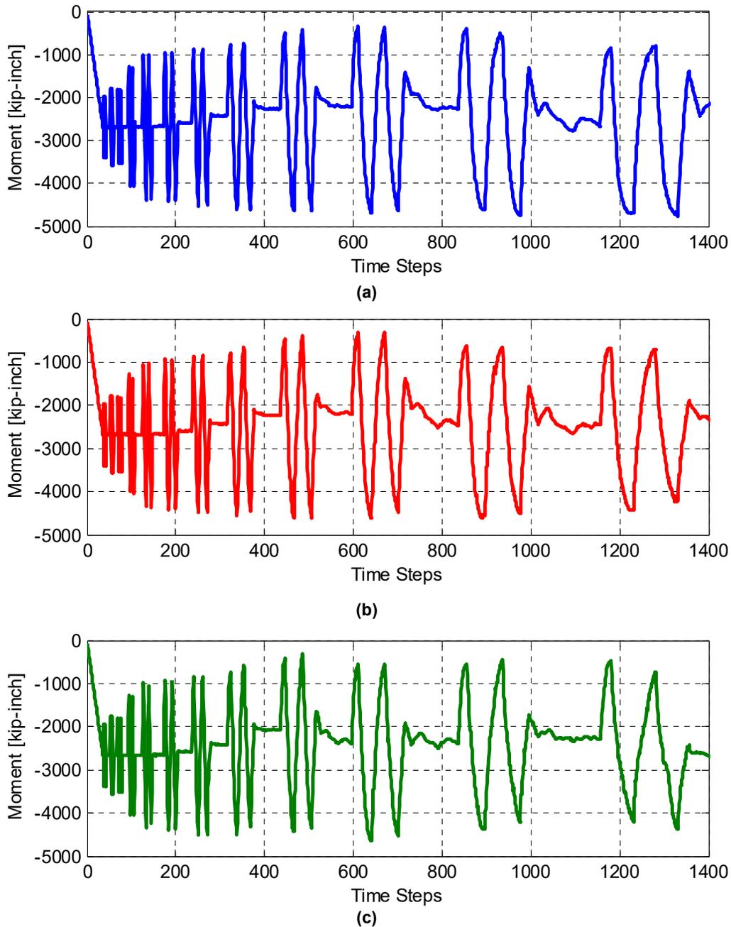
**Figure 4.26** Bent cap beam moment history at Section B from the calibrated inelastic FE model for three cases: (a) 8 #5 top and bottom original design; (b) 8 #4 top and bottom design 1; and (c) 8 #3 top and bottom design 2.
