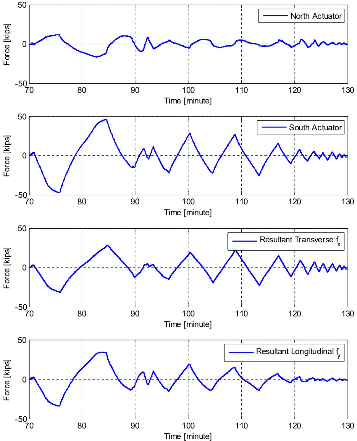
**Figure 3.18** Zoomed-in view of the history of north and south lateral actuators load cells measurements and the corresponding resultant forces in the transverse ( $f_x$ ) and the longitudinal ( $f_y$ ) directions for the 50%-scale bi-directional HS test.
