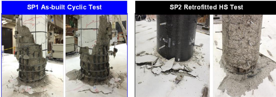
**Figure 3.88** Column plastic hinge damage after Specimen No. 1 cyclic tests and cap beam concrete crushing and column flexural cracks (observed after CFRP jacket removal) after Specimen No. 2 HS tests.
