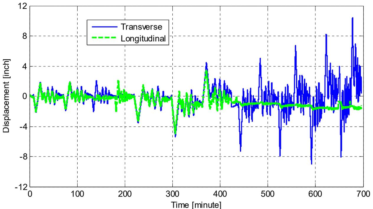
**Figure 3.10** History of the online computed (and applied) displacements in the global transverse and longitudinal directions throughout all 15 HS test runs of the retrofitted specimen (Specimen No. 2).
