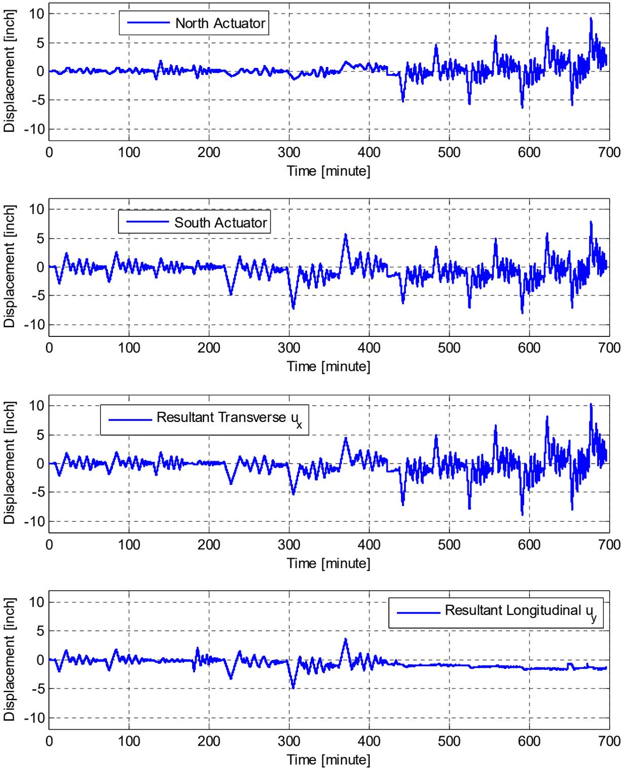
**Figure 3.11** History of north and south lateral actuators temposonics measurements and the corresponding resultant displacements in transverse ( $u_x$ ) and longitudinal ( $u_y$ ) directions for all 15 HS test runs of Specimen No. 2.
