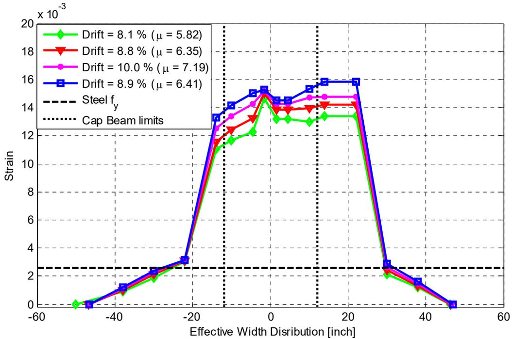
**Figure 3.69** Strain distribution in the tension side at Section B for the four large-scale transverse direction only HS test runs at the negative loading peak (expressed in terms of drift ratio and  $\mu$ ).
