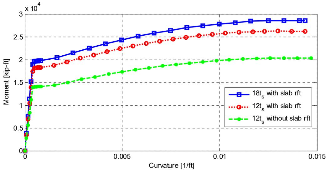
**Figure 4.41** Moment-curvature relationships for negative moment demands for the full-scale Academy Bridge three different bent cap beam cross sections as obtained from XTRACT sectional analysis results.
