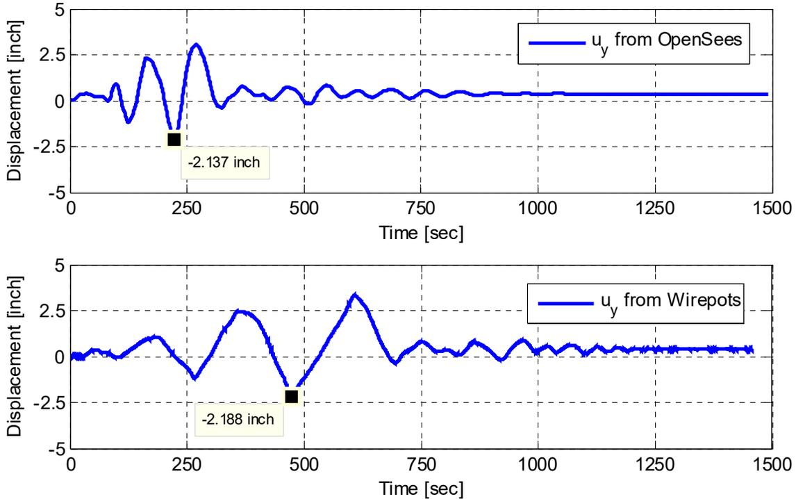
**Figure 2.39** Global longitudinal displacement history ( $u_y$ ) obtained from the OpenSees solution and that actually measured from wirepots for the repaired Specimen No. 1 80% Rinaldi bi-directional HS test.
