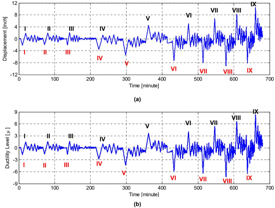
**Figure 3.63** (a) The main nine positive and negative displacement amplitudes; and (b) the corresponding ductility levels (bottom) used for investigating the effective slab width for retrofitted Specimen No. 2 tested using HS.
