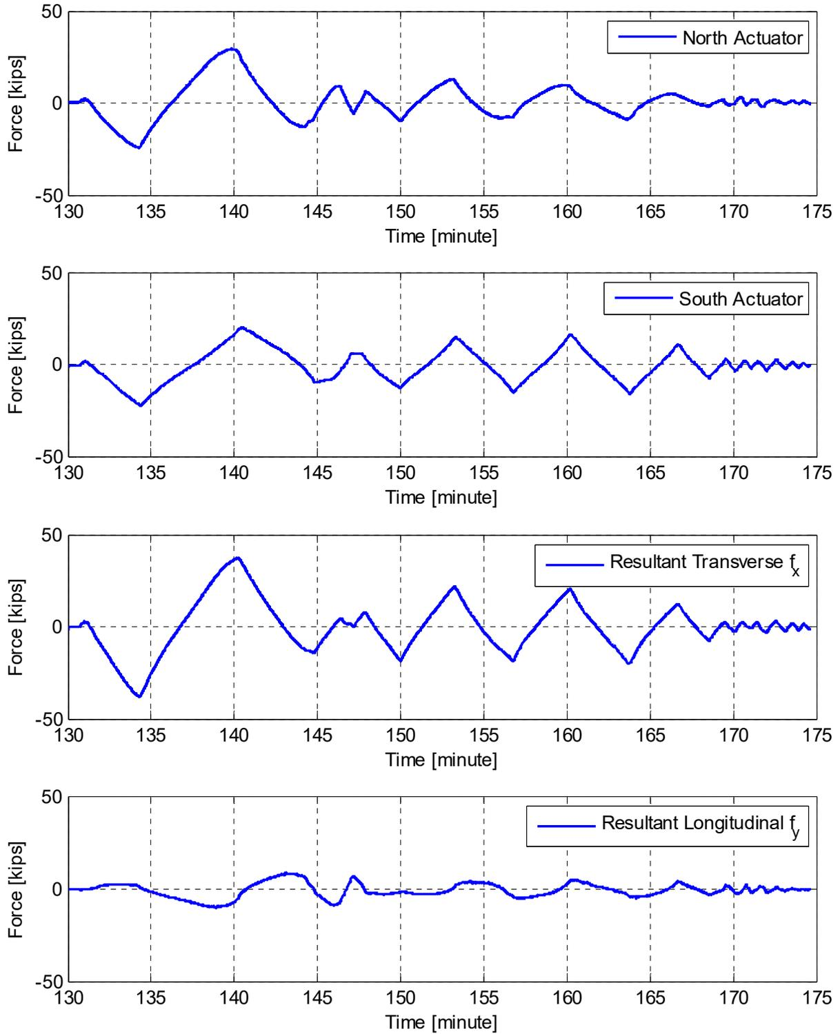
**Figure 3.19** Zoomed-in view of the history of north and south lateral actuators load cells measurements and the corresponding resultant forces in the transverse ( $f_x$ ) and the longitudinal ( $f_y$ ) directions for the 50%-scale transverse direction only HS test.
