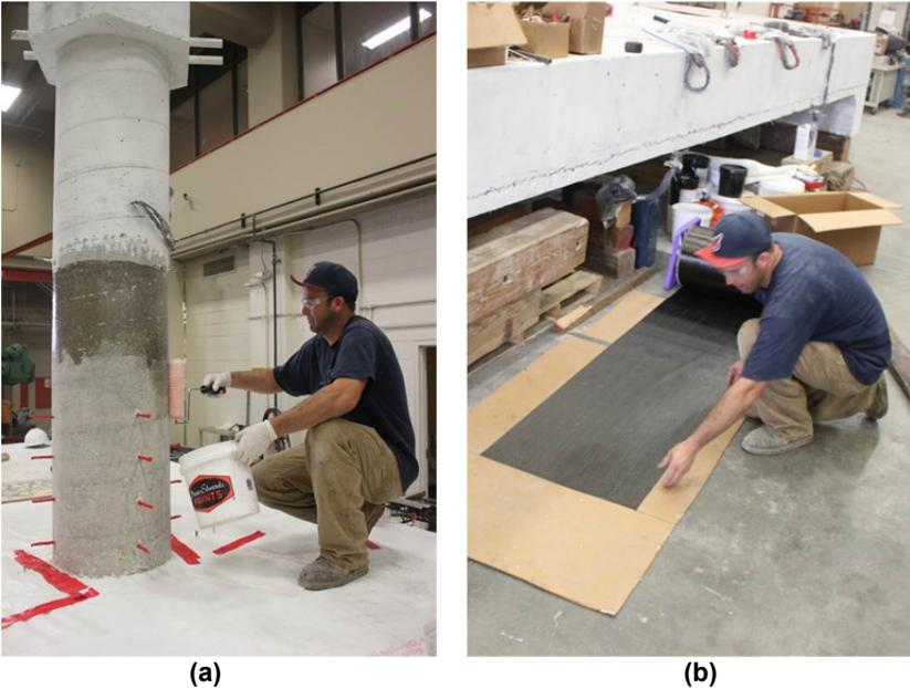
**Figure 3.2** (a) Applying a primer epoxy coat to the column surface before applying the CFRP layers; and (b) preparing a single layer of a carbon fibers sheet and cutting the sheet to the desired length.
