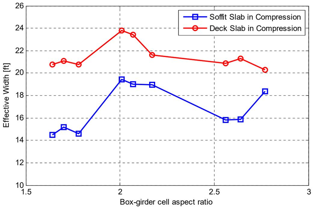
**Figure 5.23** Variation of bent cap effective width in compression at each of the soffit slab (Section 2 in Figure 5.2) and the deck slab (Section 1 in Figure 5.2) with respect to the box-girder cells aspect ratio.
