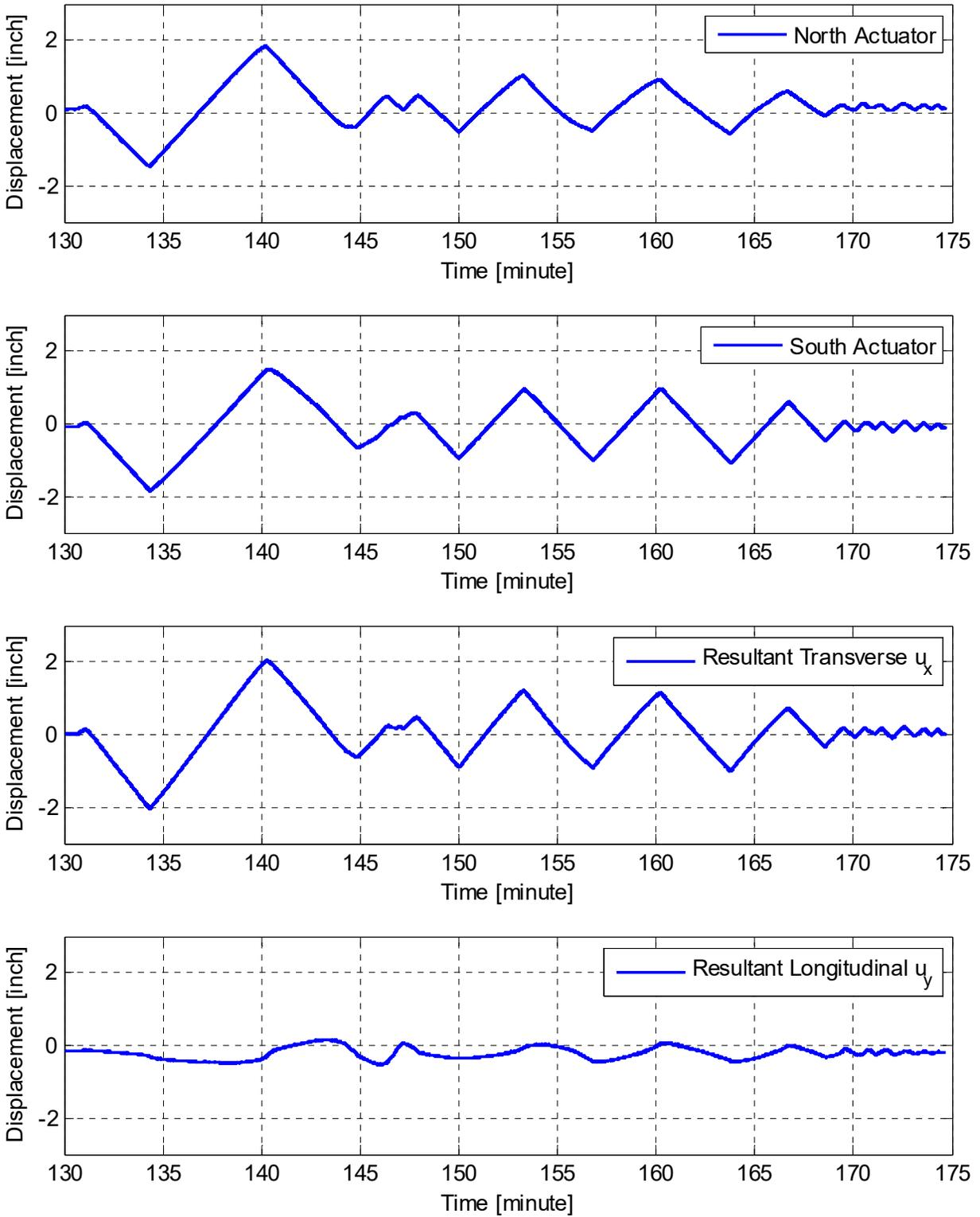
**Figure 3.13** Zoomed-in view of the history of north and south lateral actuators temponics measurements and the corresponding resultant displacements in transverse ( $u_x$ ) and longitudinal ( $u_y$ ) directions for the 50% scale transverse direction only HS test.
