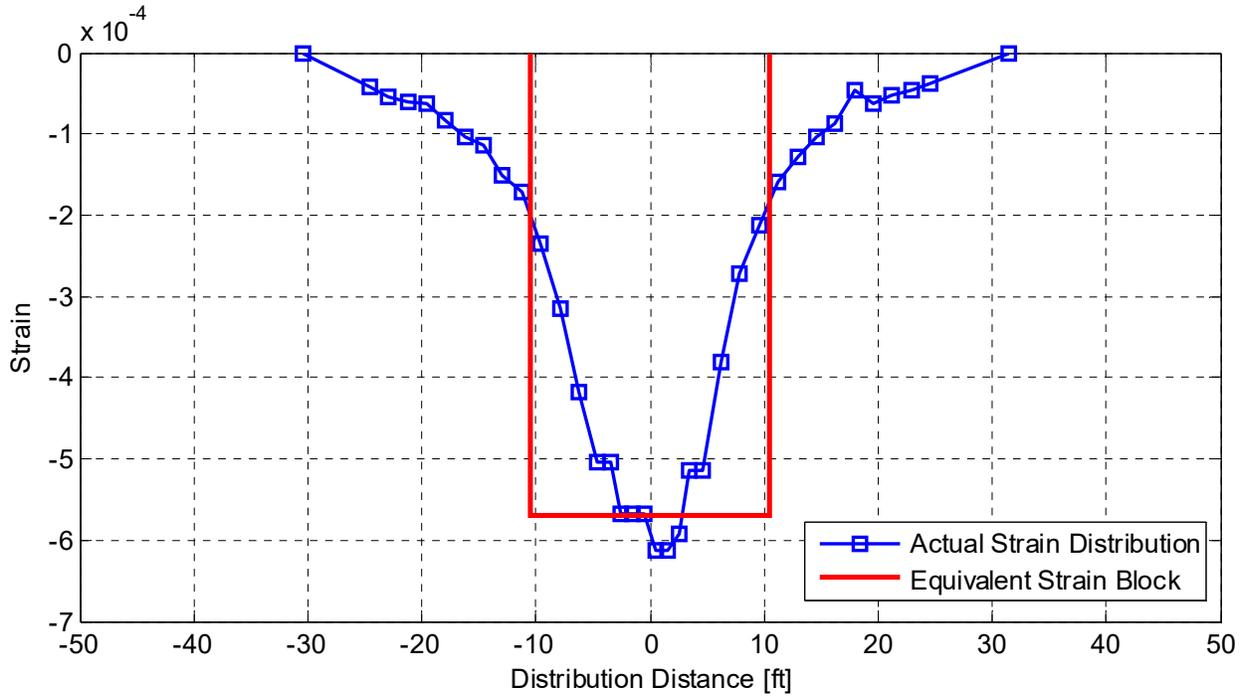
**Figure 5.7** Compression strain distribution in the bent cap and deck slab transverse reinforcement at Section 1 (identified in Figure 5.2) under combined gravity and lateral transverse load as obtained from DIANA FE linear elastic model.
