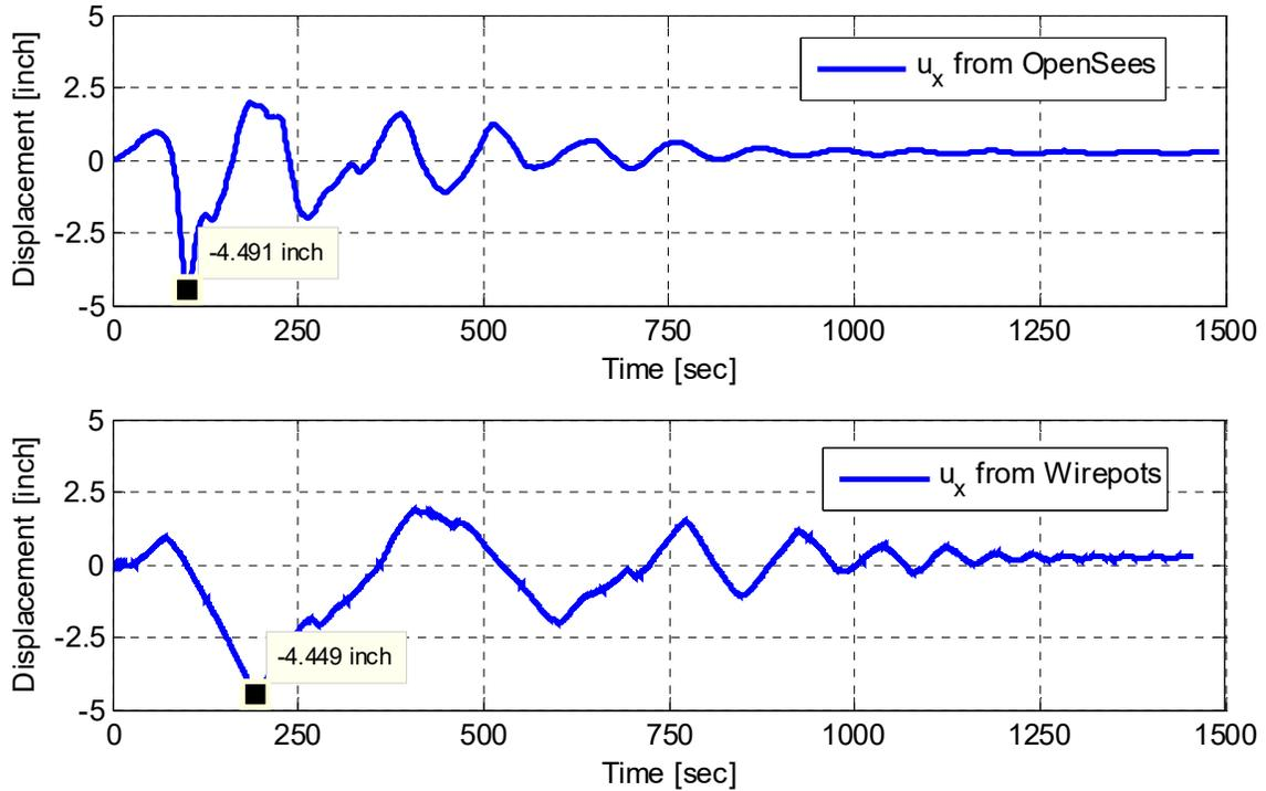
**Figure 2.38** Global transverse displacement history ( $u_x$ ) obtained from the OpenSees solution and that actually measured from wirepots for the repaired Specimen No. 1 80% Rinaldi bi-directional HS test.
