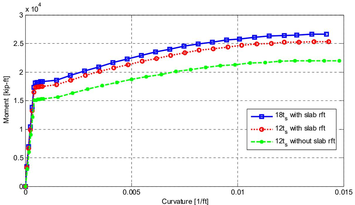
**Figure 4.40** Moment-curvature relationships for positive moment demands for the full-scale Academy Bridge three different bent cap beam cross sections as obtained from XTRACT sectional analysis results.
