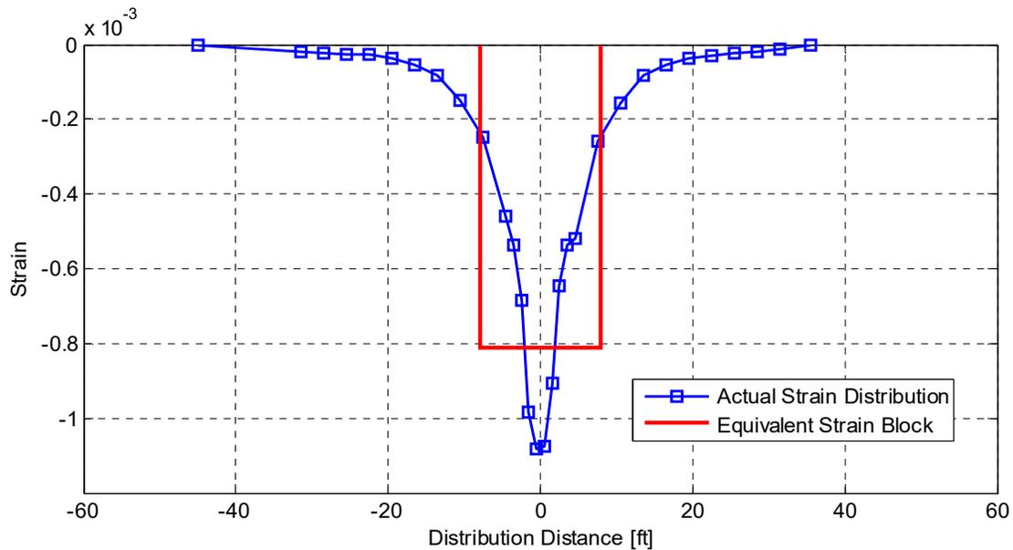
**Figure 5.9** Compression strain distribution in the bent cap and deck slab transverse reinforcement at Section 1 (identified in Figure 5.2) under combined gravity and lateral transverse load as obtained from DIANA FE linear elastic model.
