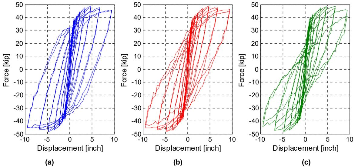
**Figure 4.24** Force-displacement relationships in the transverse direction from the calibrated inelastic FE model for three bent cap cases: (a) 8 #5 top and bottom of original design; (b) 8 #4 top and bottom design 1; and (c) 8 #3 top and bottom design 2.
