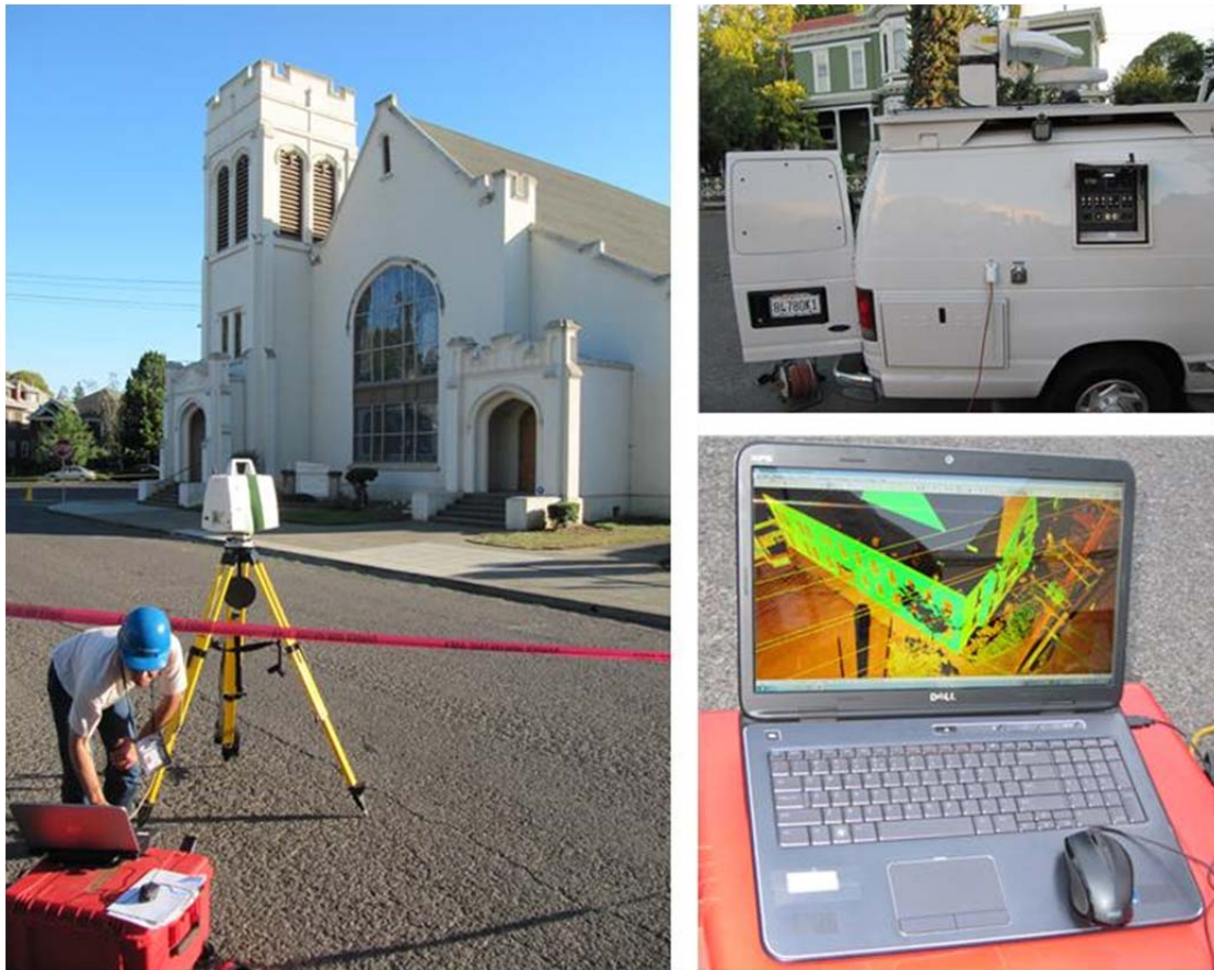
Figure 32 Laser scanner setup for historical church scan with live scanning view (bottom right) and power supplied by a TV channel especially equipped car (top right).
