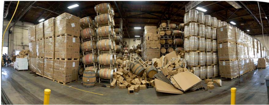
Figure 41 Panoramic view of the contents damage of the modern warehouse. Wine barrels and cases of wine bottles were stacked very high for storage and subsequently collapsed and fell during the earthquake.
