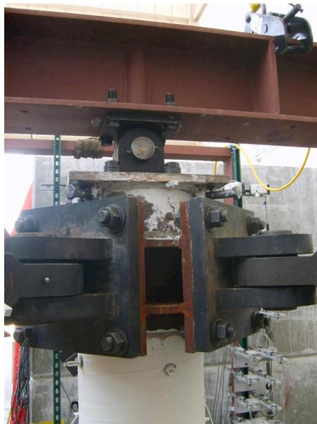
**Fig. C.9 Attachment of actuators to column.**
