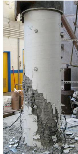
(b) Axial failure of the column
