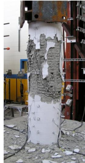
(b) Axial failure of the column
