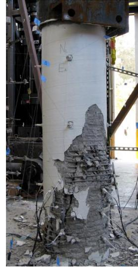
(b) Axial failure of the column
