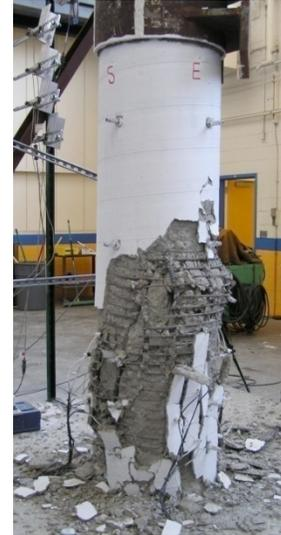
(b) Axial failure of the column
