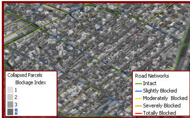
Fig. 11. Probabilistic road network blockage – part of Tehran.
