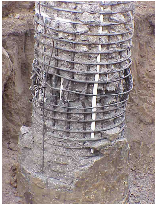
Fig. 3. Hoop fracture at maximum ductility.
