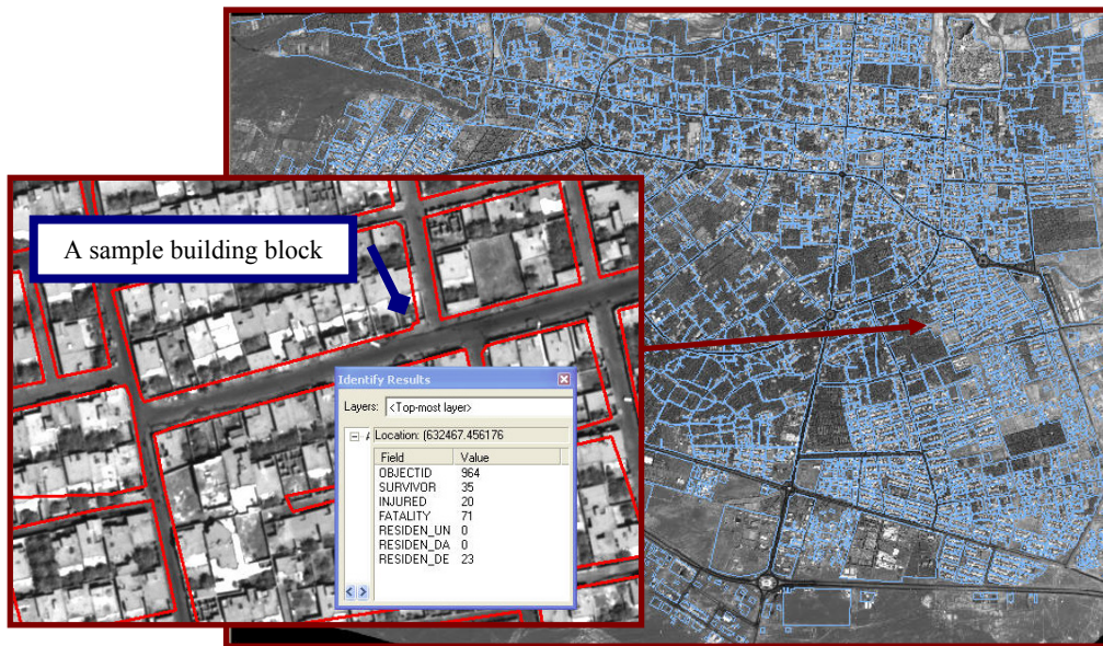
Fig. 9. BAM post disaster survey zones in GIS - overlaid on optical image (three levels of building damages in addition to three levels of human casualties).
