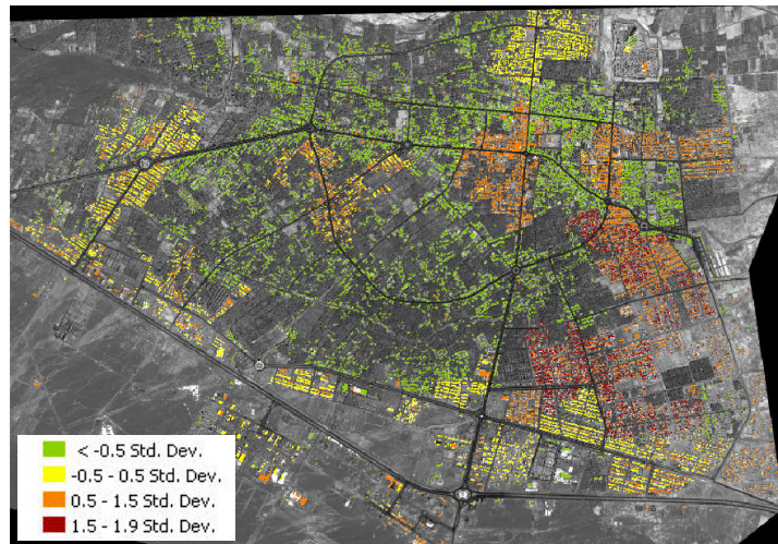
Fig. 13. Results of physical change/damage mapping in Bam using SAR data.
