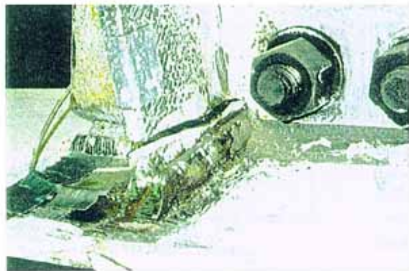
Figure 5.1.5 Fracture at Beam Top Flange, Spec. 3
