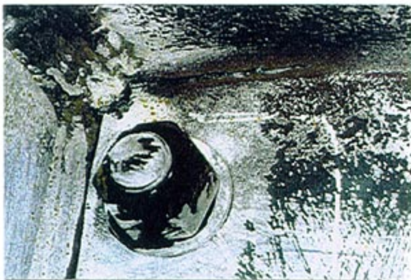
Figure 7.4.6 K-Line Slit at Beam Bottom Flange, Spec. 14
