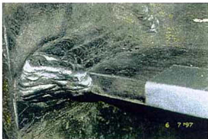
Figure 7.4.3 Overlay Weld at Bottom Flange, Spec. 14
