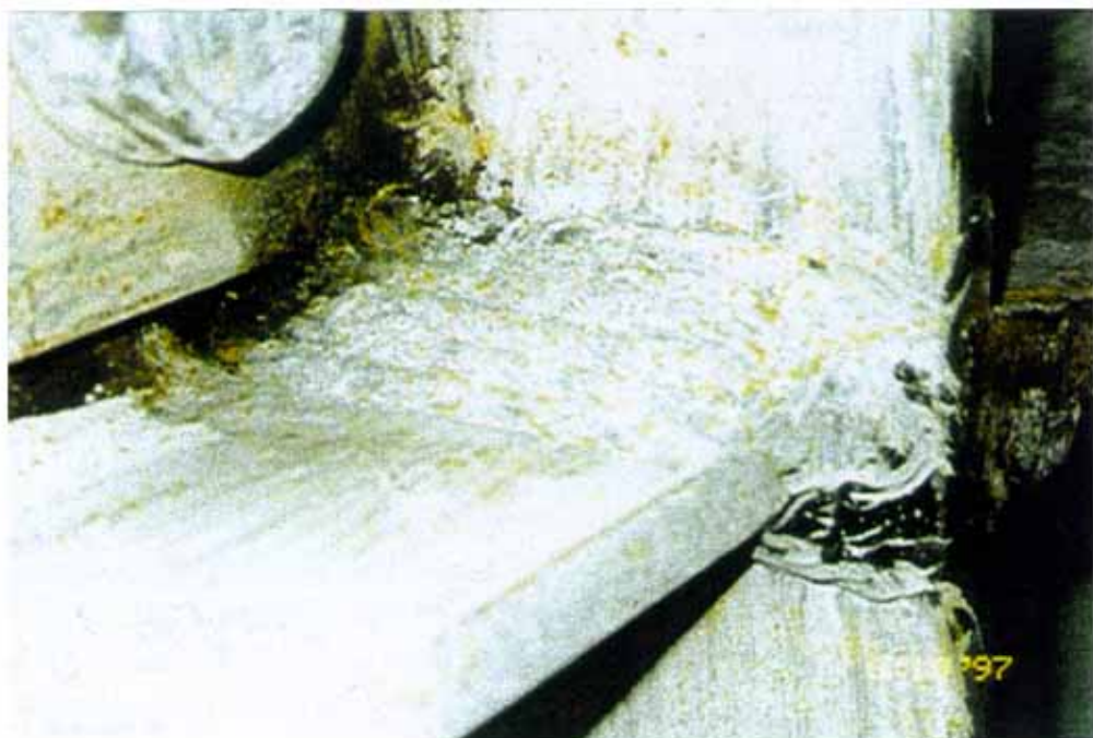
Figure 7.2.4 Overlay Weld, Bottom Flange, Spec. 10
