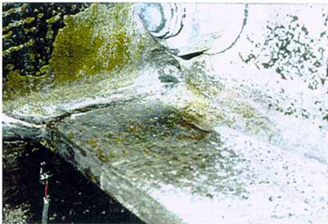
Figure 4.2.2 Repaired Bottom Flange Weld, Spec. 1R
