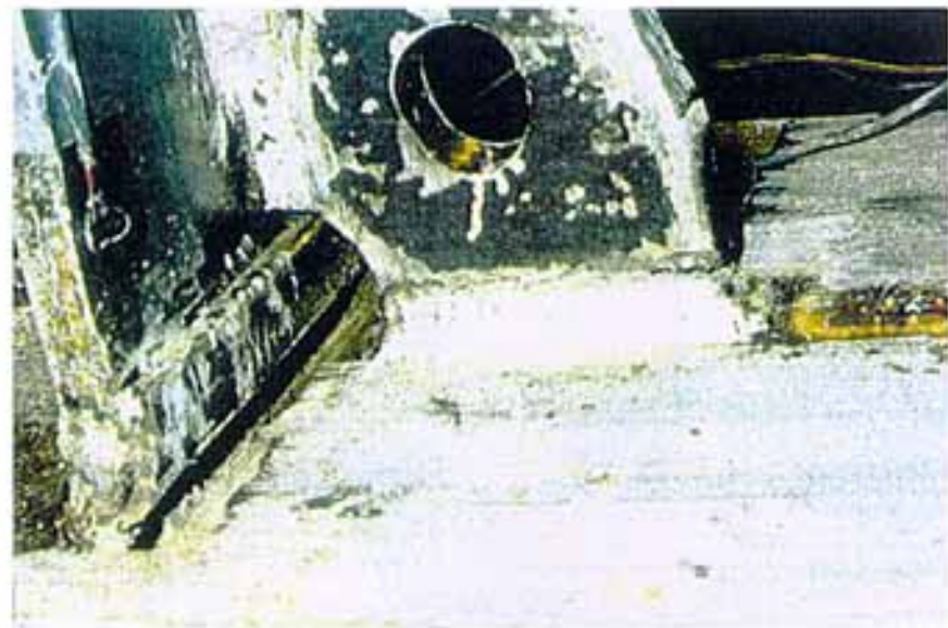
Figure 5.3.4 Pullout at Beam Bottom Flange, Spec. 6
