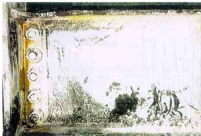
Figure 4.2.5 Plastic Hinge in Beam, 1R
