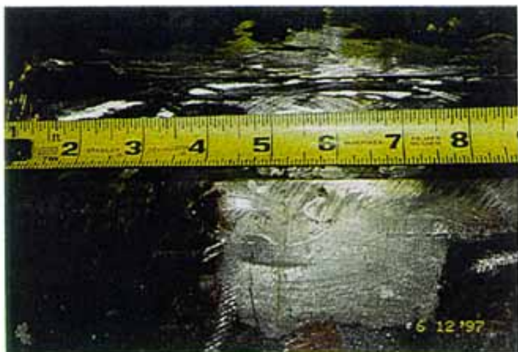
Figure 7.2.3 Gouged Out Bottom Side, Bottom Flange, Spec. 10
