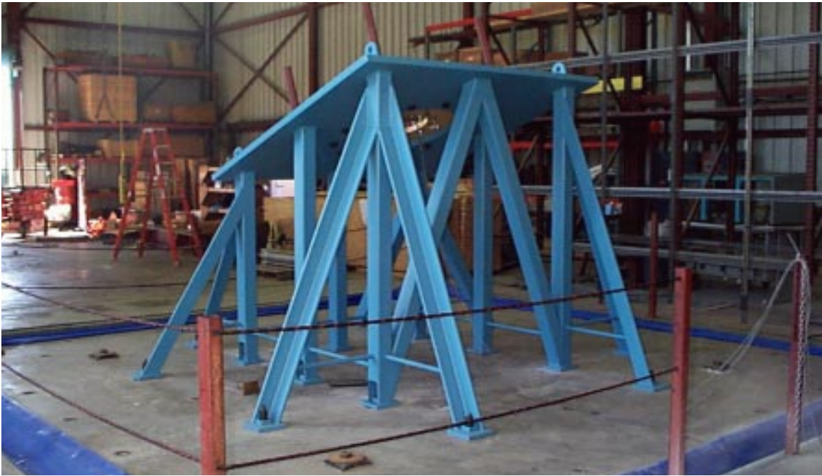
a. View of the mounting frame showing angle braces
