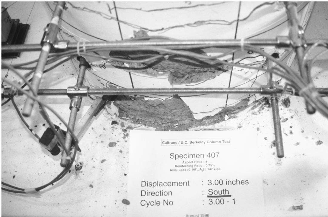
**Figure 3.9: Column 407 Spalled Region at 3-Inch Displacement Level**
