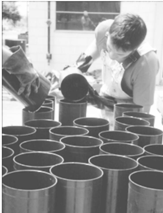
**Figure A.14: Casting Concrete Cylinders**
