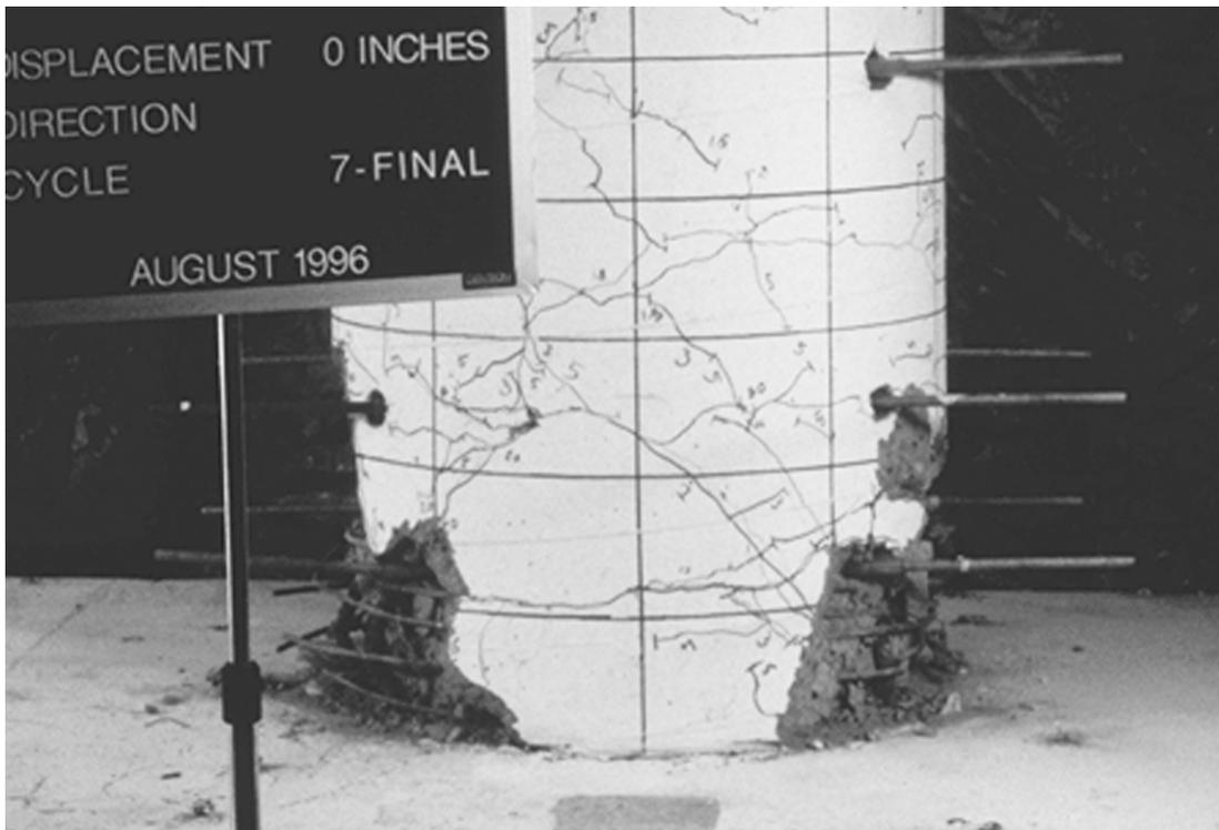
**Figure 3.13: Column 407 Final Damage State**
