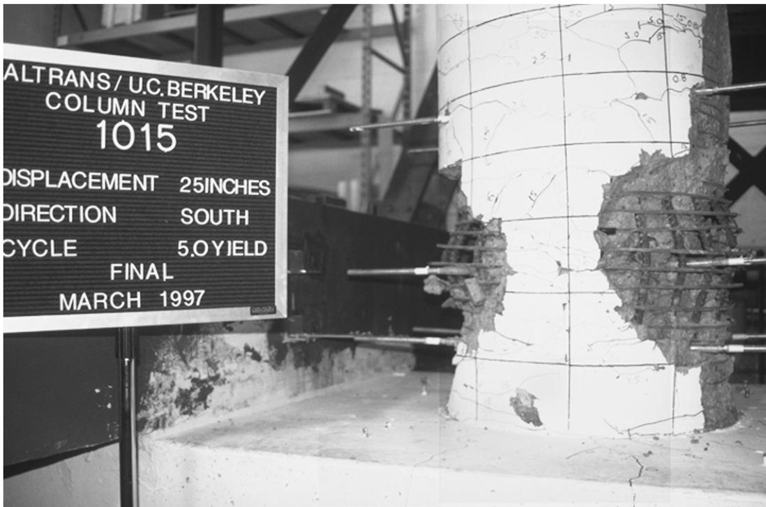
**Figure 3.38: Column 1015 Damage State after Testing**
