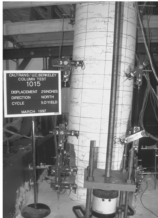
**Figure 3.37: Column 1015 Displaced to 25 Inches**
