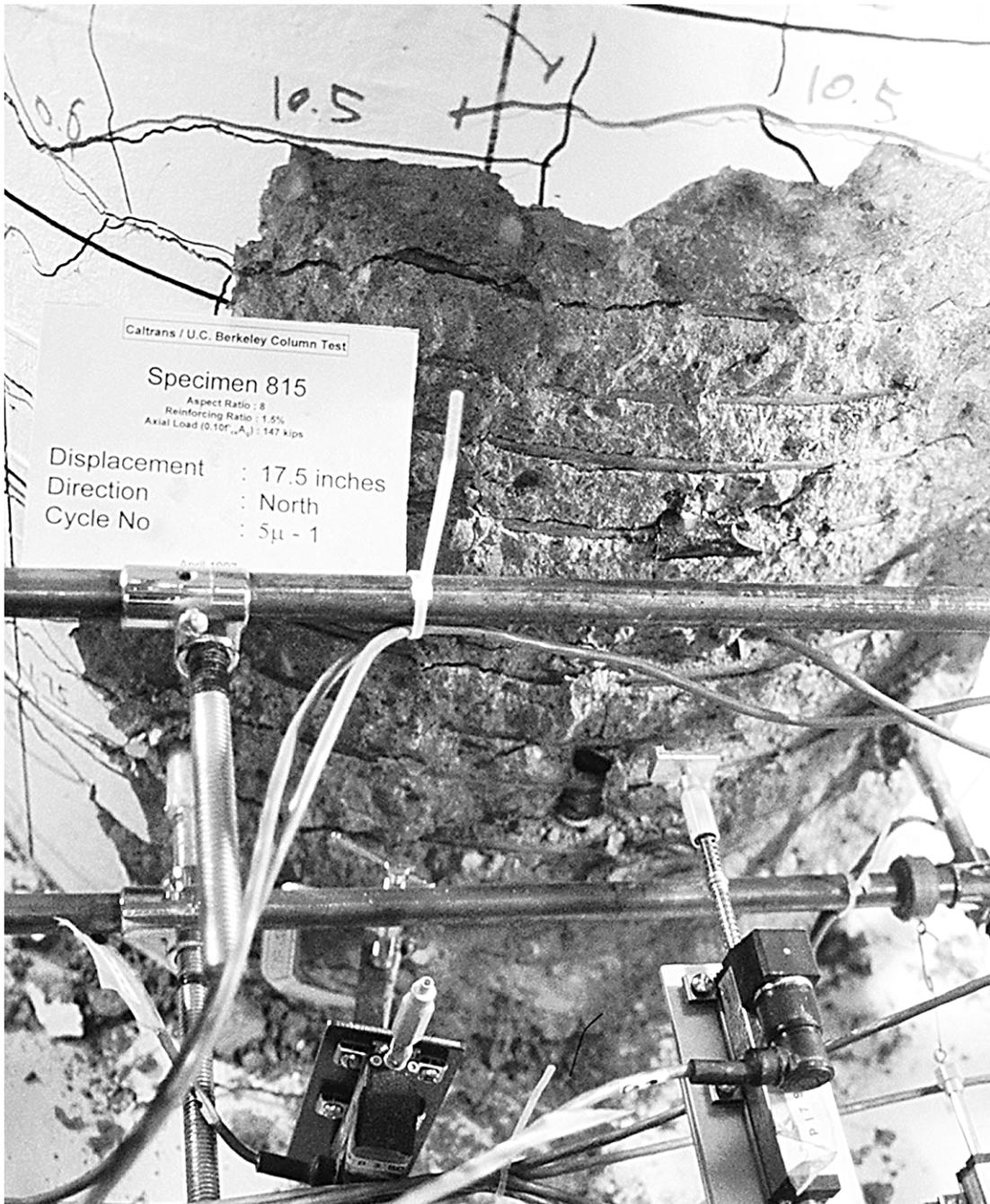
**Figure 3.27: Column 815 Spalled Region at First Cycle to 17.5 Inches**
