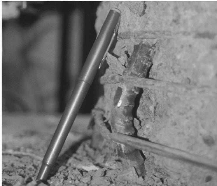
**Figure 3.10: Column 407 Buckled Bar and Fractured Spirals**
