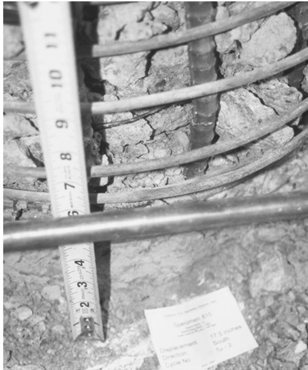
**Figure 3.28: Column 815 Fracture of Previously Buckled Longitudinal Bar**
