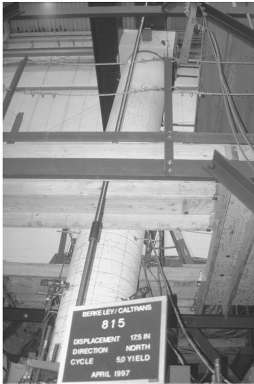
**Figure 3.30: Column 815 Displaced to 17.5 Inches**
