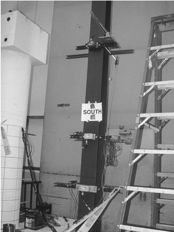
**Figure B.8: Instruments Attached to the Reference Column**
