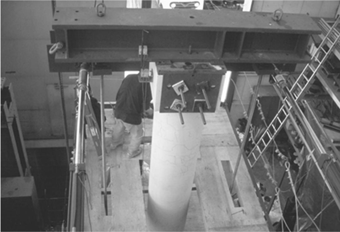
**Figure B.7: Actuators Used for Testing of Columns 815 and 1015**
