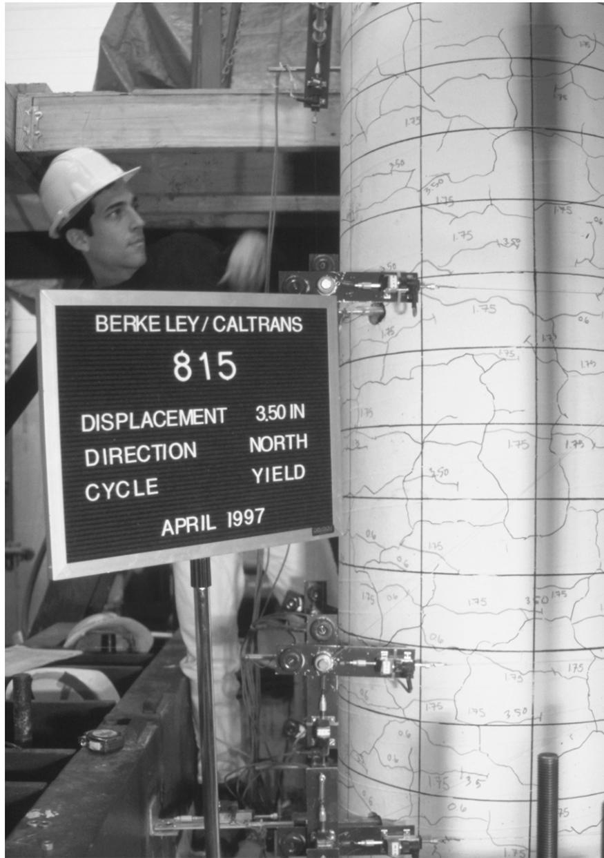
**Figure 3.26: Column 815 Crack Pattern at 3.5-Inch Displacement Level**
