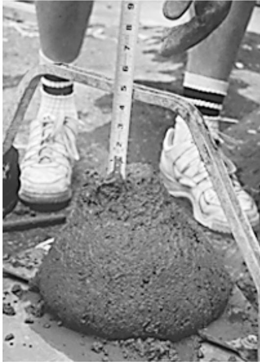
**Figure A.13: Slump Test**
