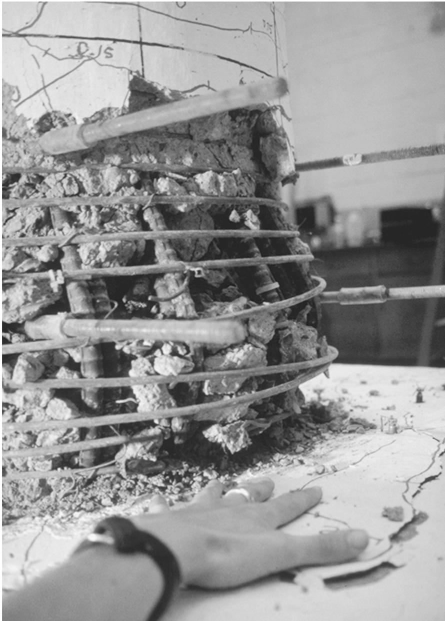
**Figure 3.23: Column 430 Final Damage State**
