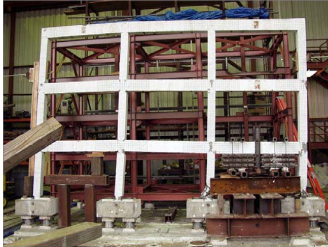
Figure 1.8 Shaking table test to validate models for simulating collapse of nonductile concrete frame. Right-hand portion collapsed onto restraining frame.
