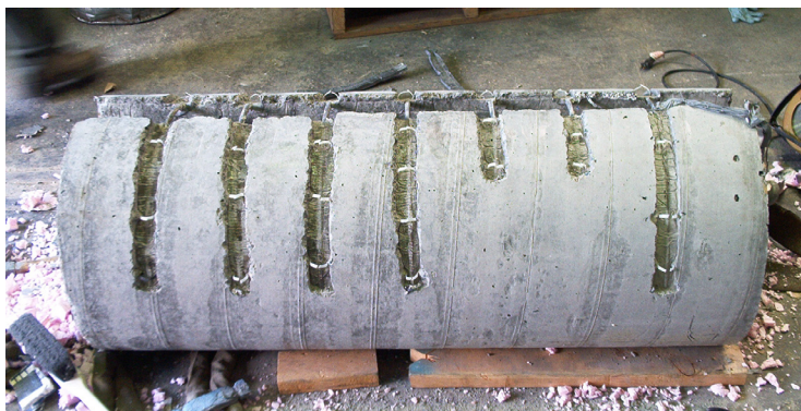
Figure 1 - Hoop stiffness test specimens.
