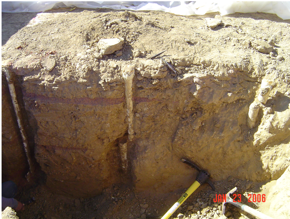
Figure 2: Failure plane from abutment test.
