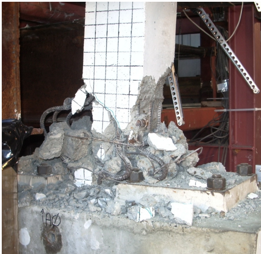
Column collapse in three-story frame test
