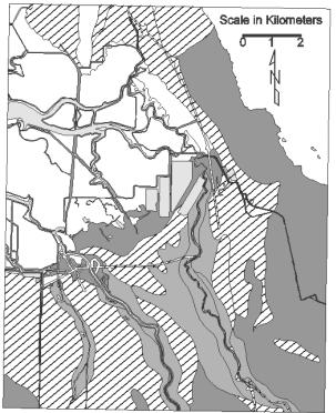
Fig. 2. Liquefaction-induced ground settlement (ft), Milpitas 7.5-minute Quadrangle, California (settlement calculated using Wu et al., 2003 method)
