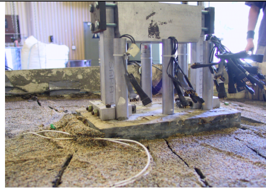
(b) Centrifuge pile group with passive bulge & lateral spreading.
