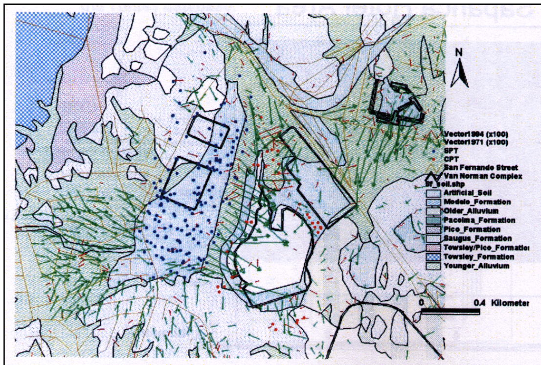
Figure 34. Typical GIS output from lateral spread case history database showing spread displacement vectors and boring locations. (Bardet, 2002 [58])
