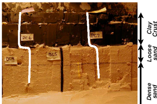
Figure 3-15: Excavation of SJB02 showing the strong localized deformation at the interface between the loose sand and overlying clay layer (paper markers highlighted for clarity). Note that the clay is dark and the horizontal black seam in the sand is a colored marker separating the loose and dense layers.
