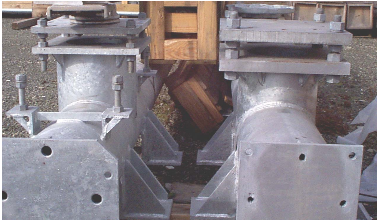
Fig. 4.6. Difference in base design for Original (left) and Modified (right) Switches
