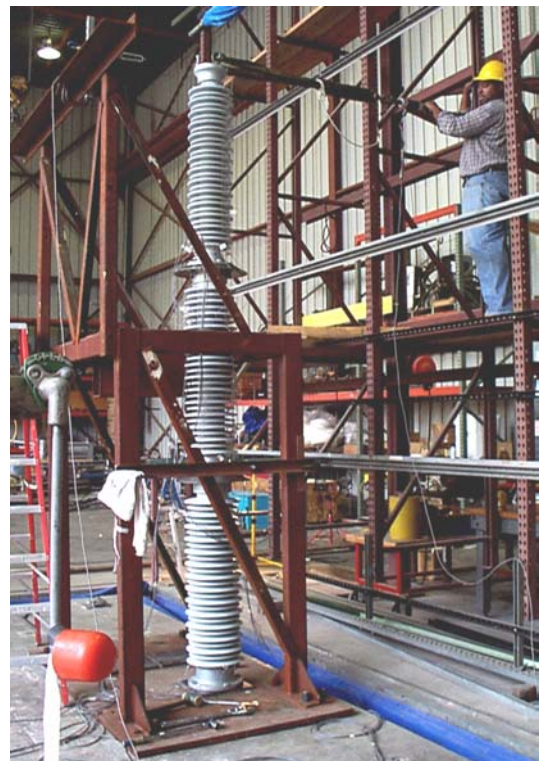
Fig. 3.2. Test setup for insulator post testing: drawing (left) and test in progress (right).
