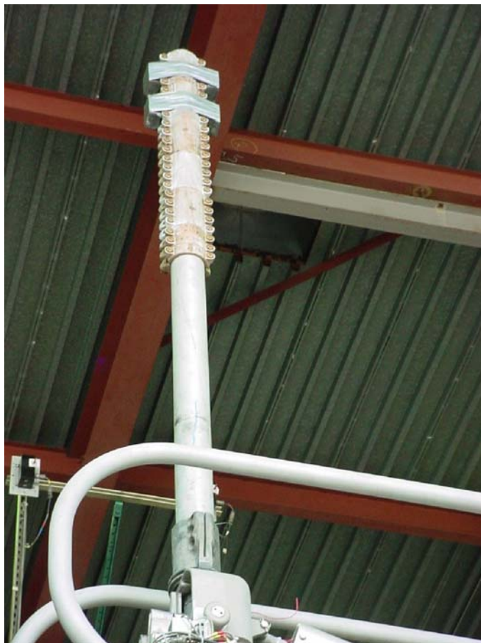
Fig. 7.3 Shortened blade installed in the switch.
