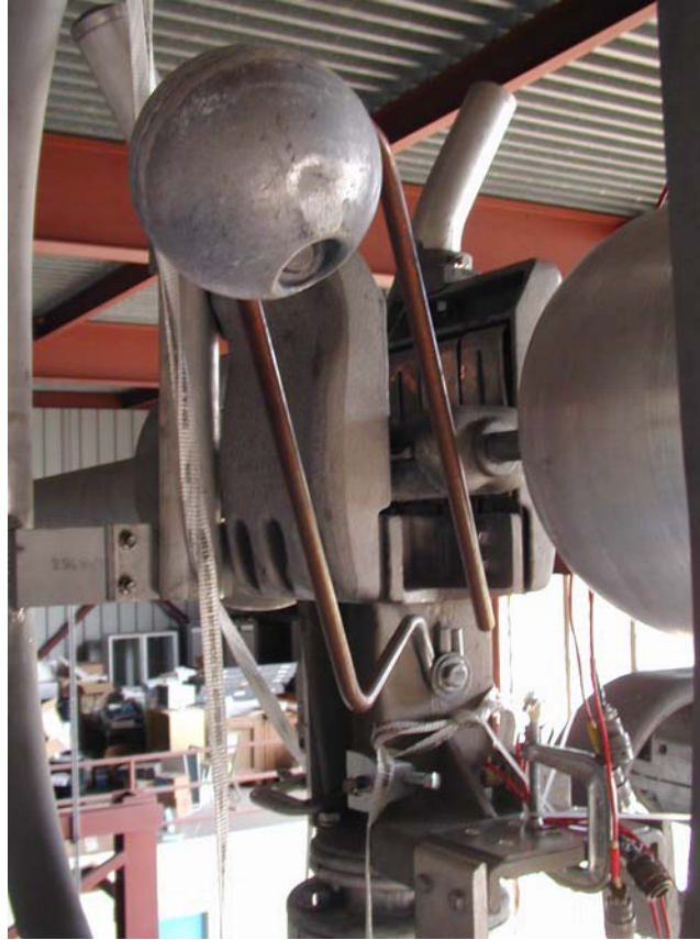
Fig. 5.9 Anomaly 1: stationary arc horn bent away from blade (used to be in contact with blade).
