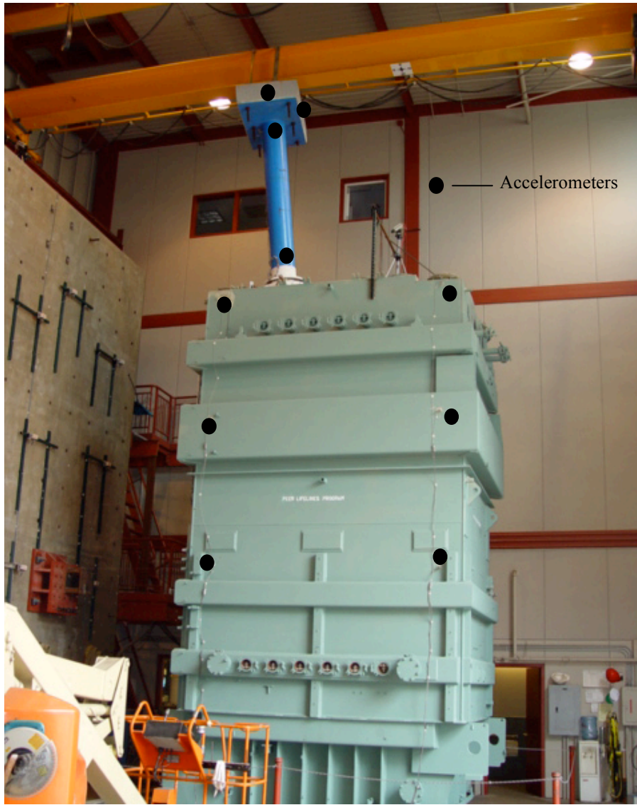
Figure 5.8 – Accelerometers Locations on East Face of Transformer Tank
