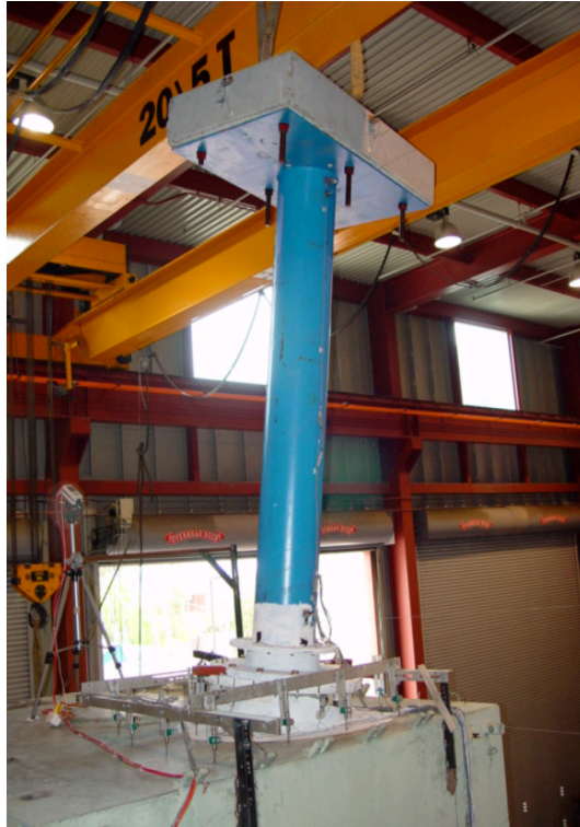
Figure 5.7 - Mock Bushing Assembly Attached to Top of Transformer Tank.
