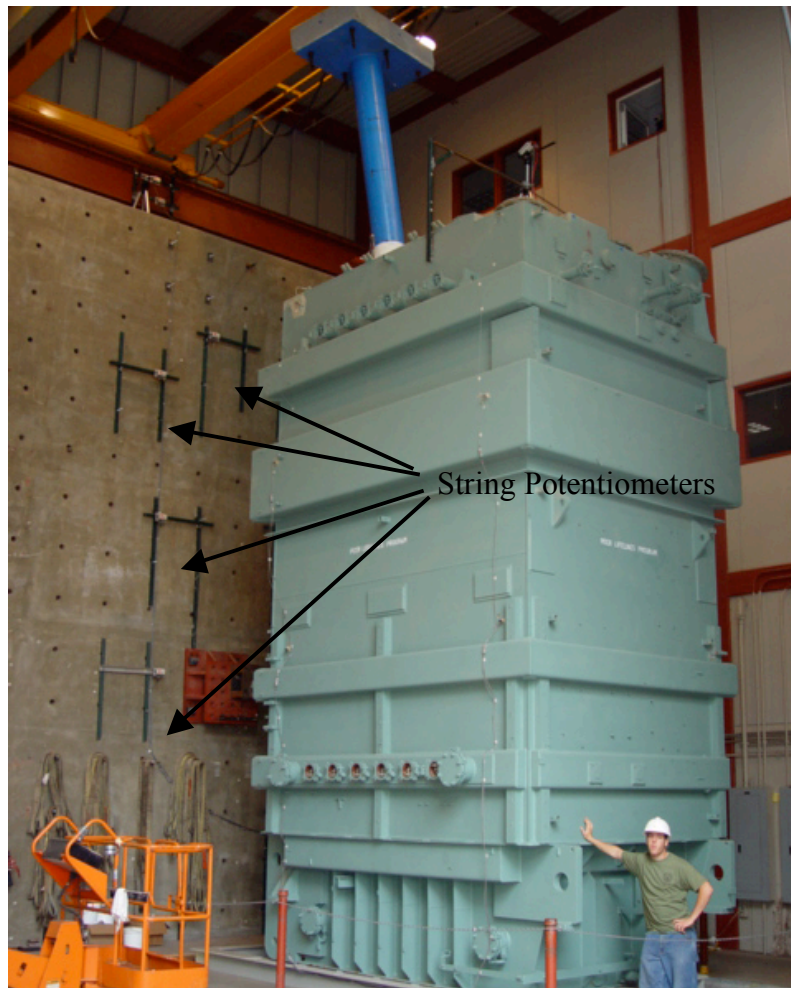
Figure 5.11 - Strong Wall and Horizontal String Potentiometers.
