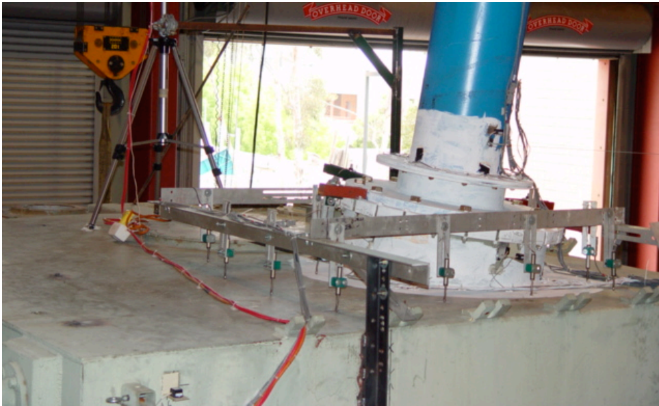
Figure 5.9 - Displacement Transducers Measuring the Out of Plane Displacement of the Top Plate.
