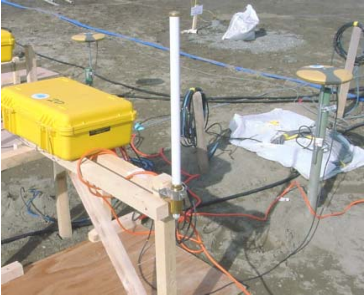
Figure 7 – Typical field unit with equipment enclosure (left), wireless transceiver antenna (center), and GPS antenna (right).
