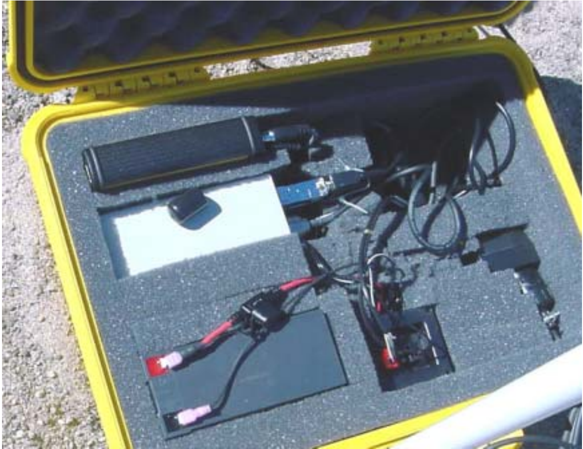
Figure 6 – Equipment enclosure housing the GPS receiver, wireless equipment, and backup power system
