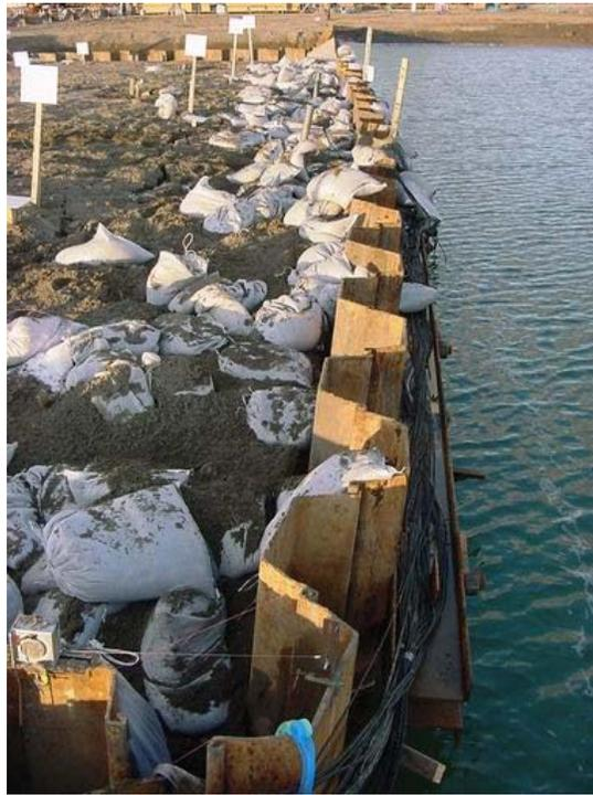
Figure 4.101 Movement of Quay Wall after the Test
