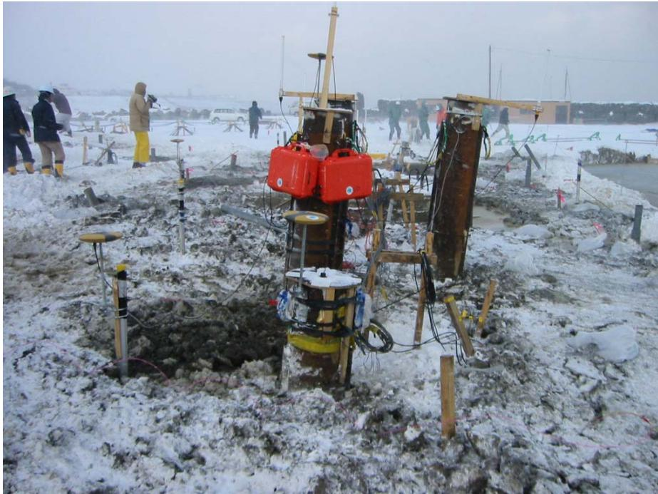
Figure 5.86 Tilting of Group of Single Piles
