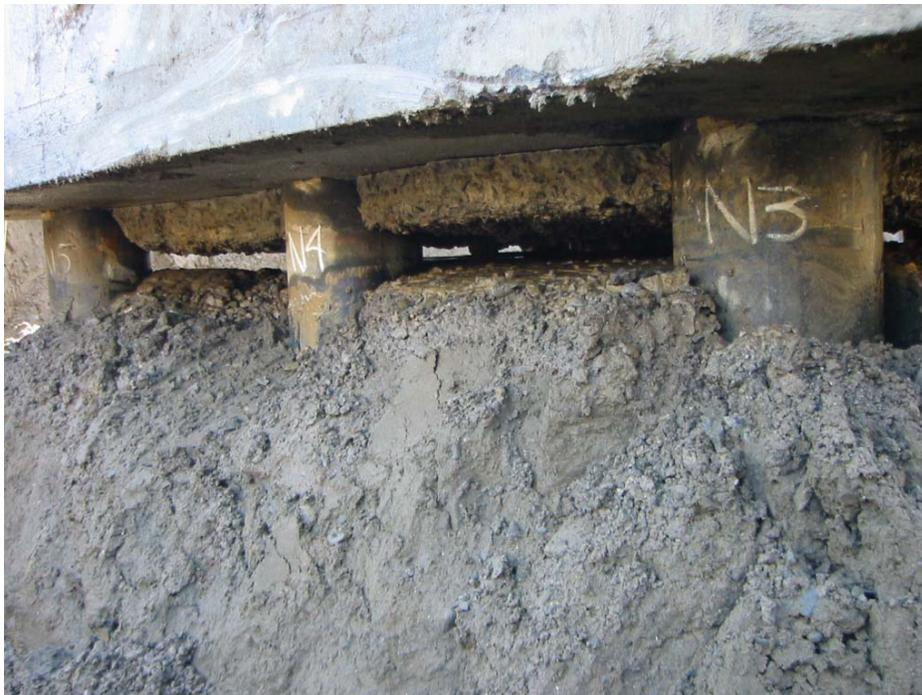
Figure 5.92 Condition of Piles to Pile Cap Connection of 9-Pile Group after Lateral Spread
