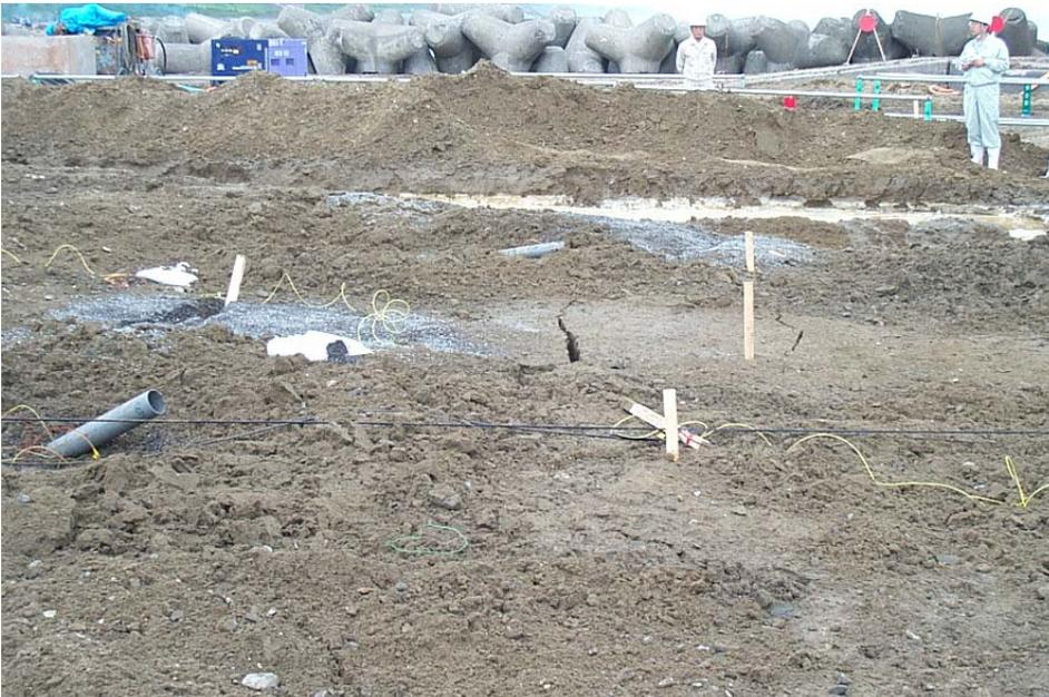
Figure 2.25 Surface Cracks after the Blast
