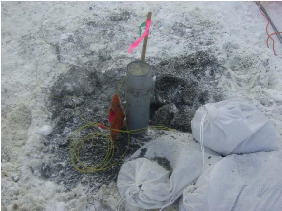
Figure 5.88 Water Coming from Inclinometer Casing
