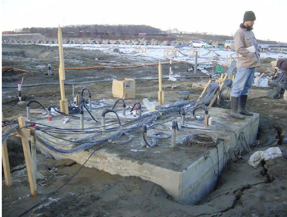
Figure 5.4 Site Condition before 2<sup>nd</sup> Blast Test Showing Settlement and Gapping around 9-Pile Group
