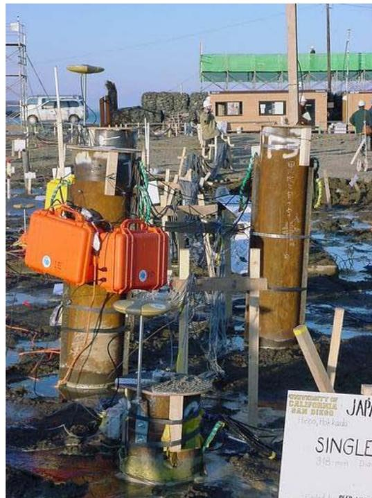
Figure 4.102 Permanent Rotation of Single Piles
