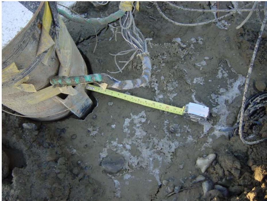
Figure 5.5 Site Condition before 2<sup>nd</sup> Blast Test Showing Gapping around Single Pile
