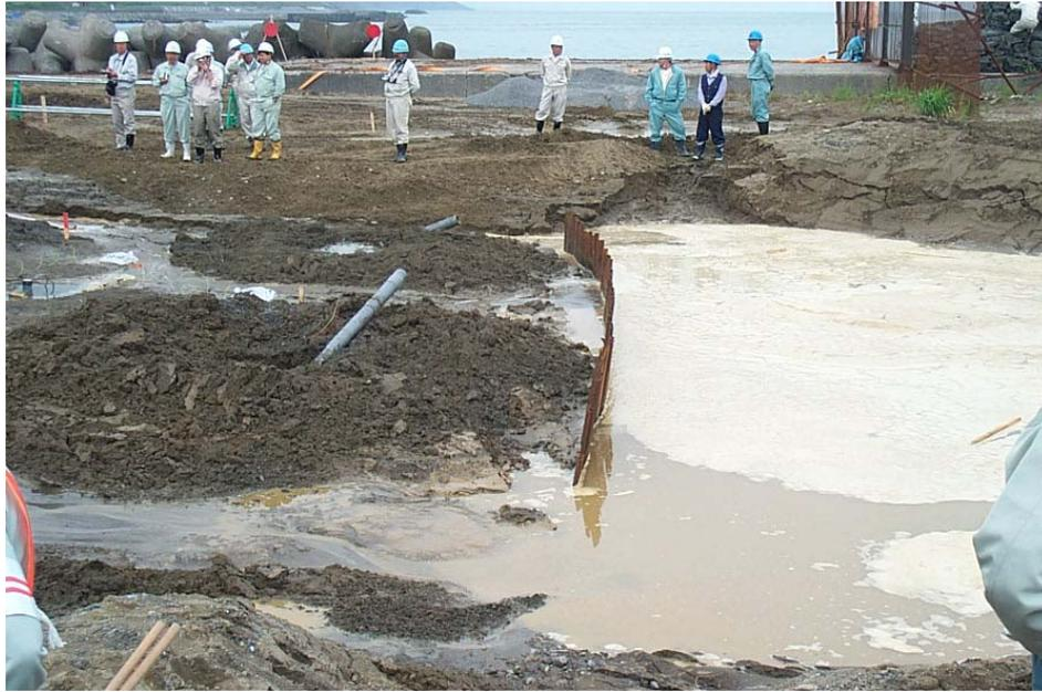
Figure 2.24 Movement of Sheet Pile Wall following Blasting
