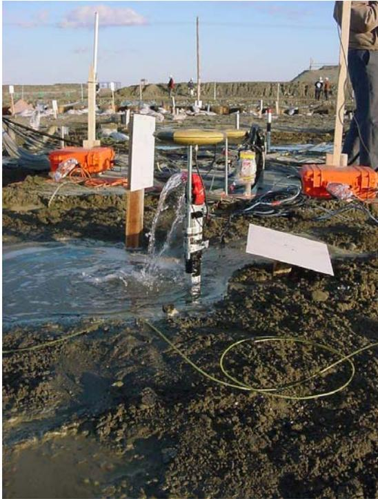
Figure 4.106 Water Coming from Inclinometer Casing
