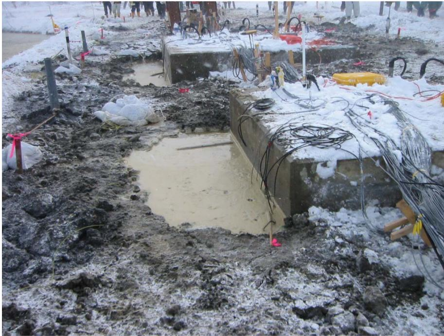
Figure 5.85 Settlement and Water Pond on Downstream Side of Pile Groups
