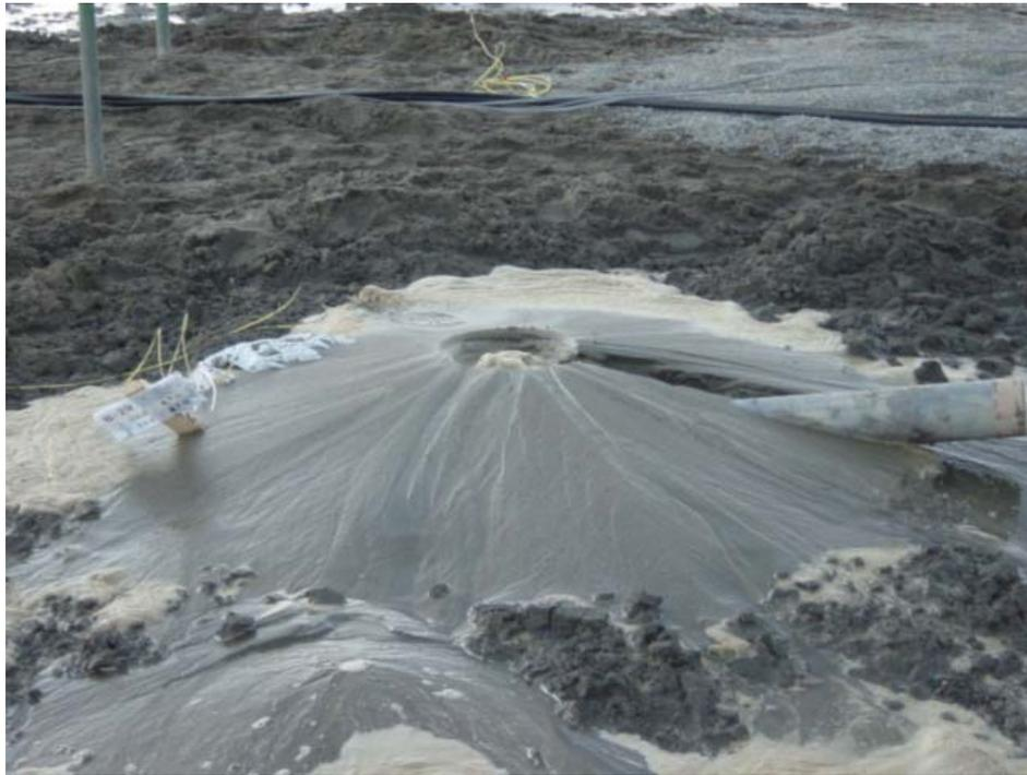
Figure 4.105 Sand Boils Following Blasting in Vicinity of Soil Embankment
