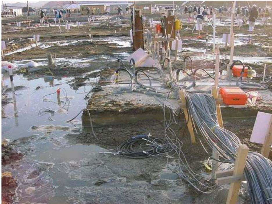
Figure 4.103 Settlement around 9-Pile Group after Blasting
