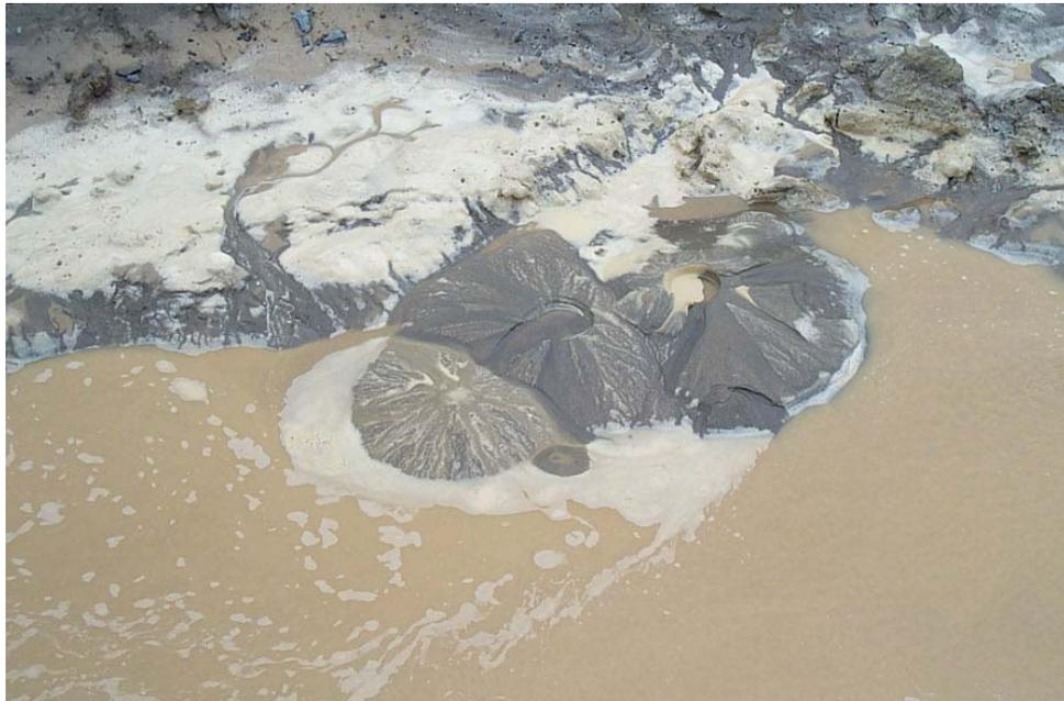
Figure 2.27 Evidence of Liquefaction : Sand Boils
