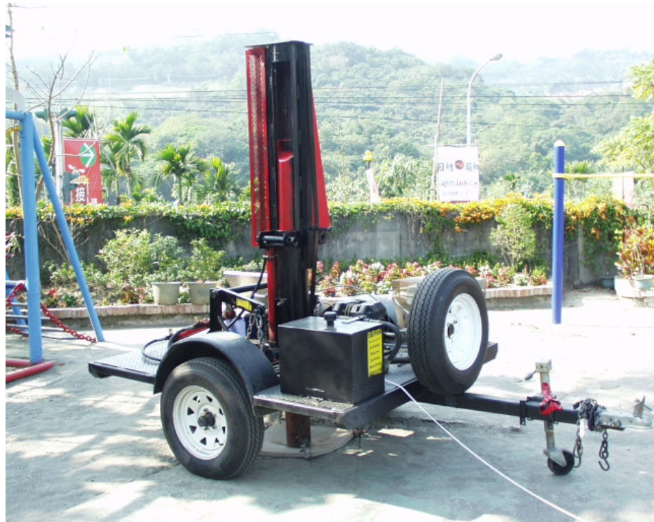
Figure 10 DynaSource Used as Impact Source at Kung-Chung Elementary School Site (TCU-52)
