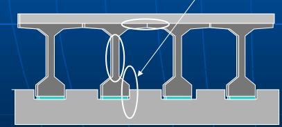
Contact of a PC girder to stopper results in failure of lower flange, shear failure of web plate, rupture of deck slabs and connection between deck slab and upper flange
