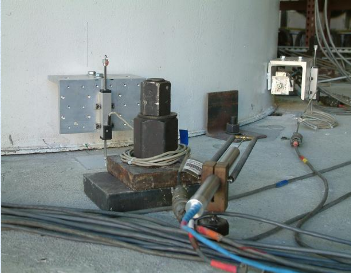
DCDT's, Linpots and 3-component accelerometers are installed around the base of the tank.
