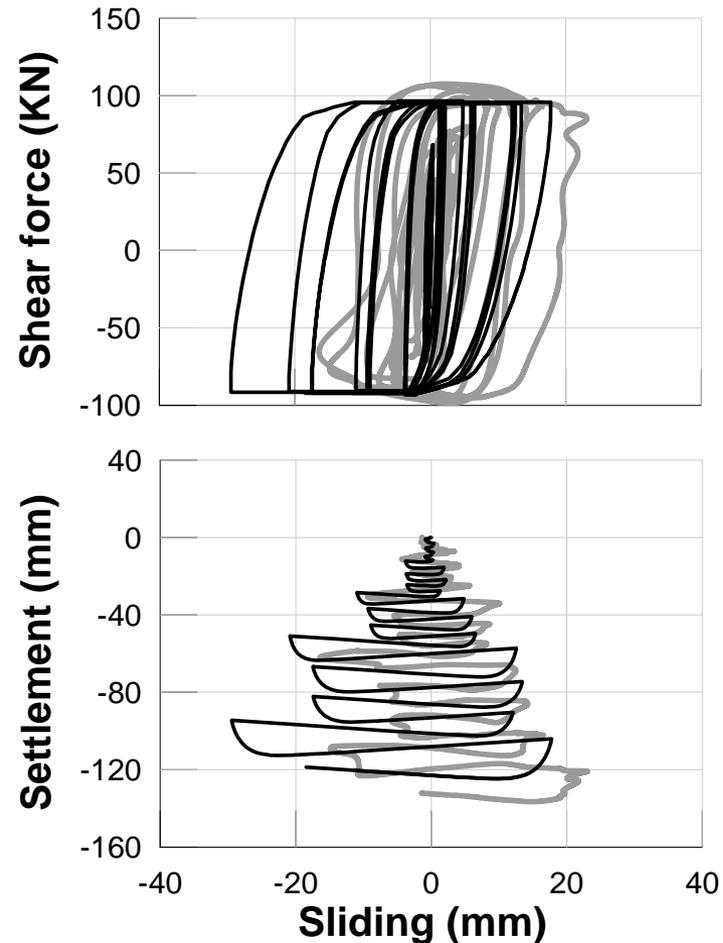
**SSG02\_05 centrifuge test ( $Dr = 80\%$ ,  $FS_v = 2.6$ ,  $M/(H \times L) = 1.72$ )**
