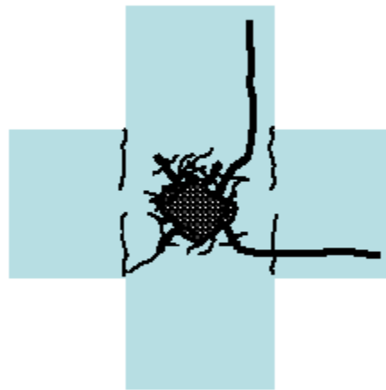
(a) Distribution of cracking and spalling
