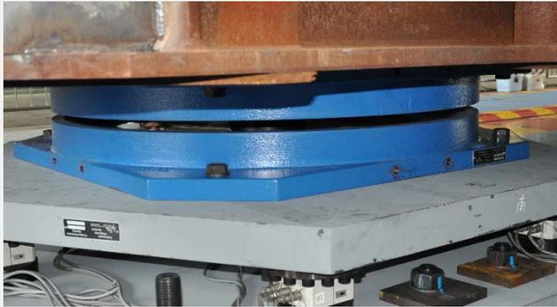
**Isolated with hybrid configuration of lead-rubber and cross-linear bearings**
