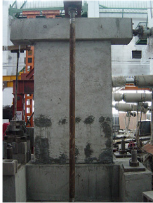
Fig. 17. Test setup for RC shear wall specimen.
