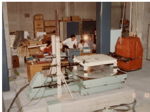
Photo 1. and Photo 2. Tiny seismic isolated structure with heavy iron weight
