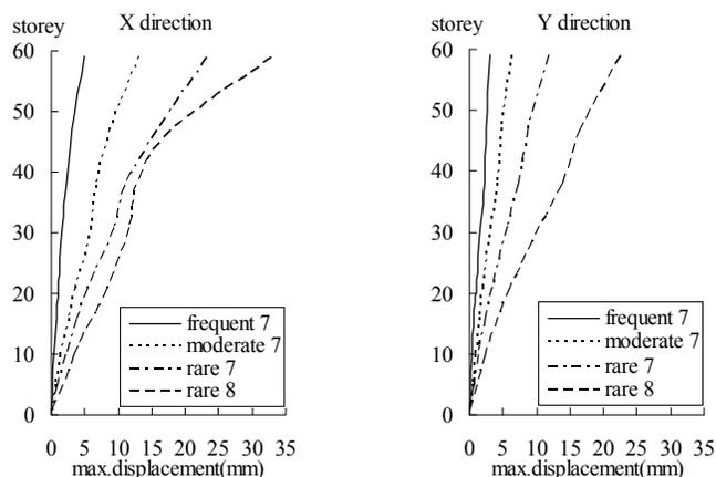
**Fig. 9 Displacement response envelopes of the model structure**
