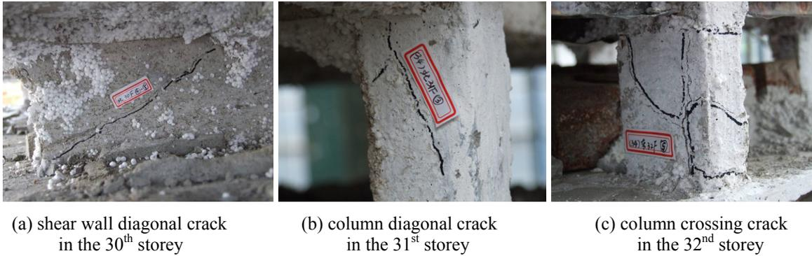
**Fig. 7 Failure pattern of the model structure**
