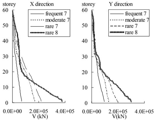
**Fig. 10 Envelopes of the shear force**
