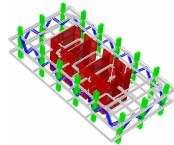
**Fig. 2 Belt truss in the 47<sup>th</sup> floor**
