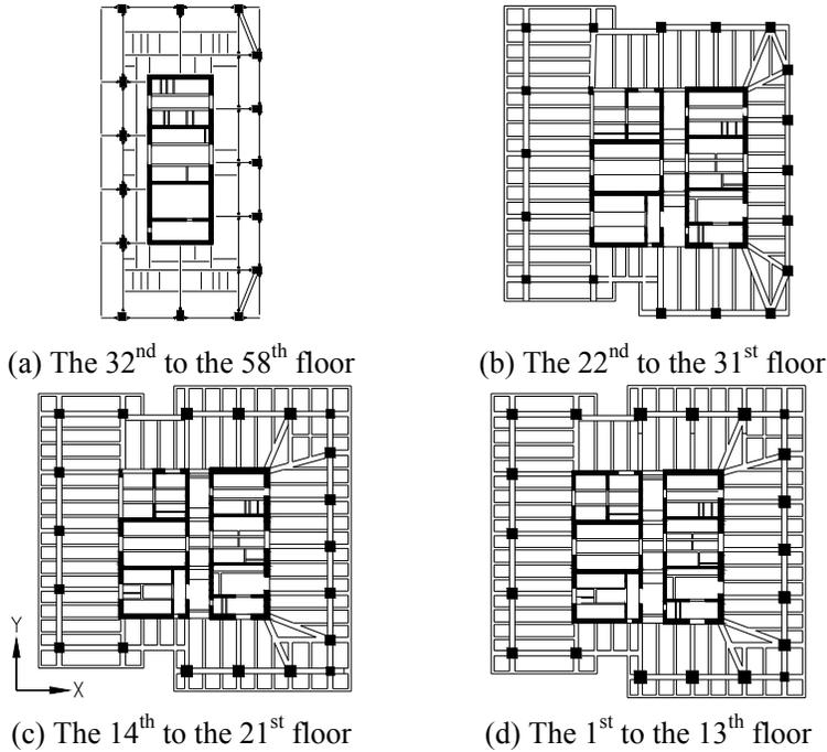
**Fig. 1 Typical plan layouts of each part**
