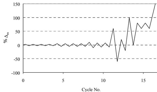
(h) Wood - CUREE Near Fault (Kraw. et al., 2000-b)
