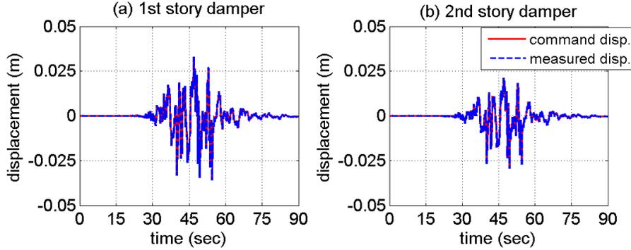
**Fig. 5. Comparison of command and measured actuator displacements**
