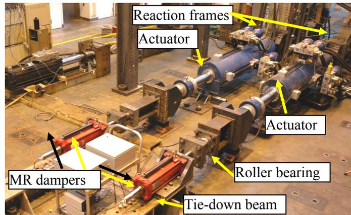
**Fig. 3. Experimental setup for real-time hybrid simulation**
