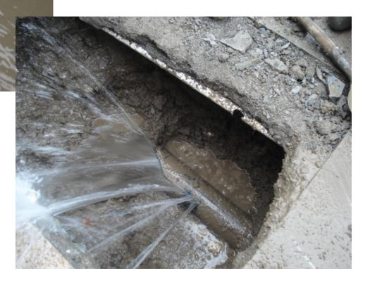
Damage to PVC pipeline
