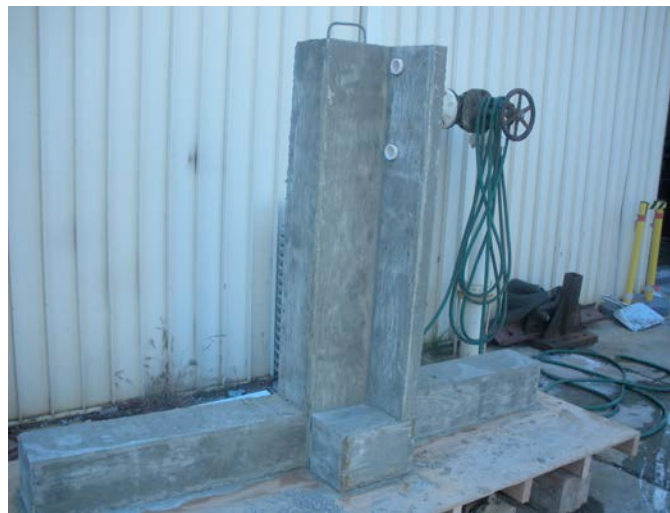
Figure 3.23: Specimen after removing the form
