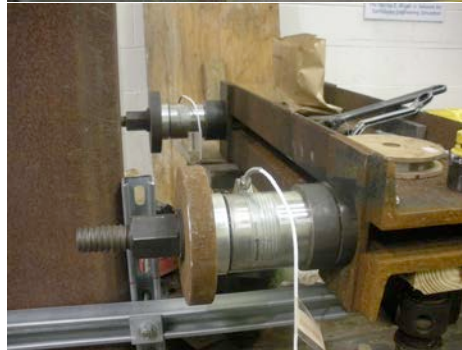
Figure 4.11: Compression measuring load cells
