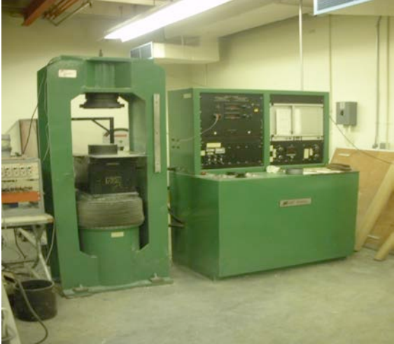
Figure 3.4: Compression machine used to test concrete cylinders
