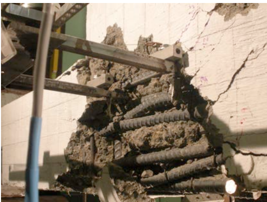
Figure 5.6: Damage progression leading to collapse
