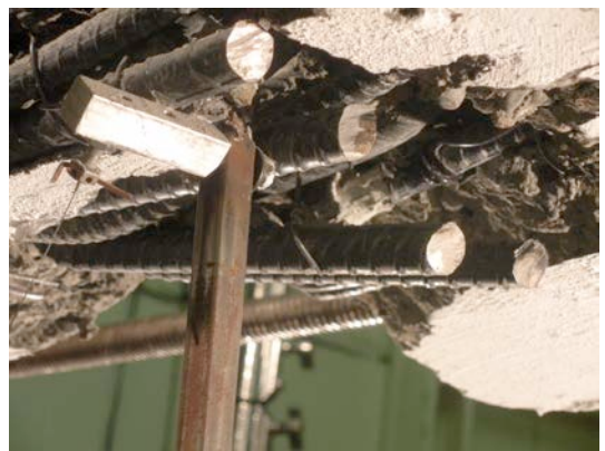
Figure 5.6: Damage progression leading to collapse
