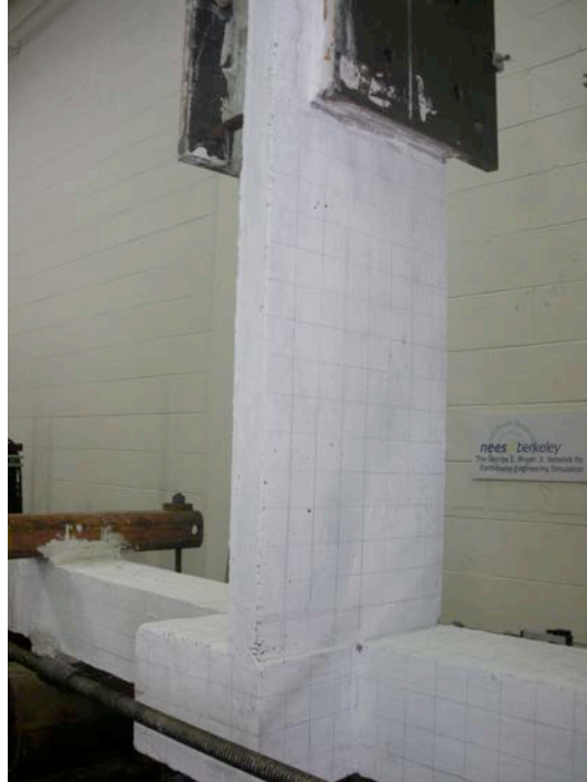
Figure 3.24: Grid lines on the specimen
