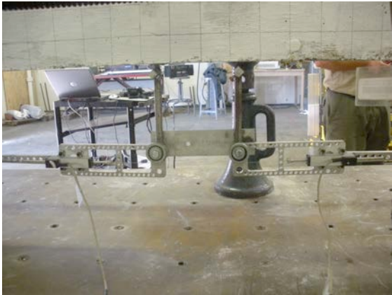
Figure 4.3: Displacement transducers- shear strain on bottom of joint
