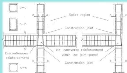
**Figure 2: Insufficient Detailing.**
