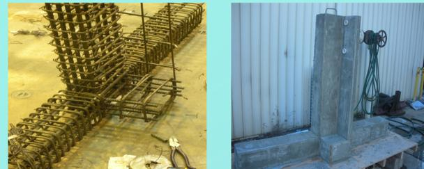
**Figure 3: Test Specimen.**
