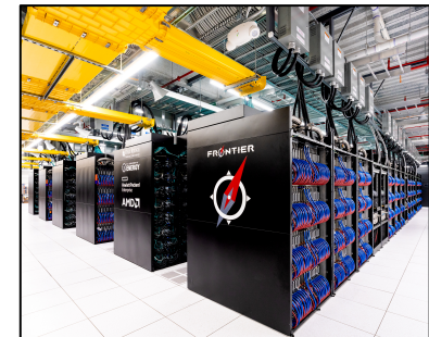
Frontier, 2022, GPU-accelerated 1,102 Pflop/s Top500 #1 Oak Ridge National Lab
