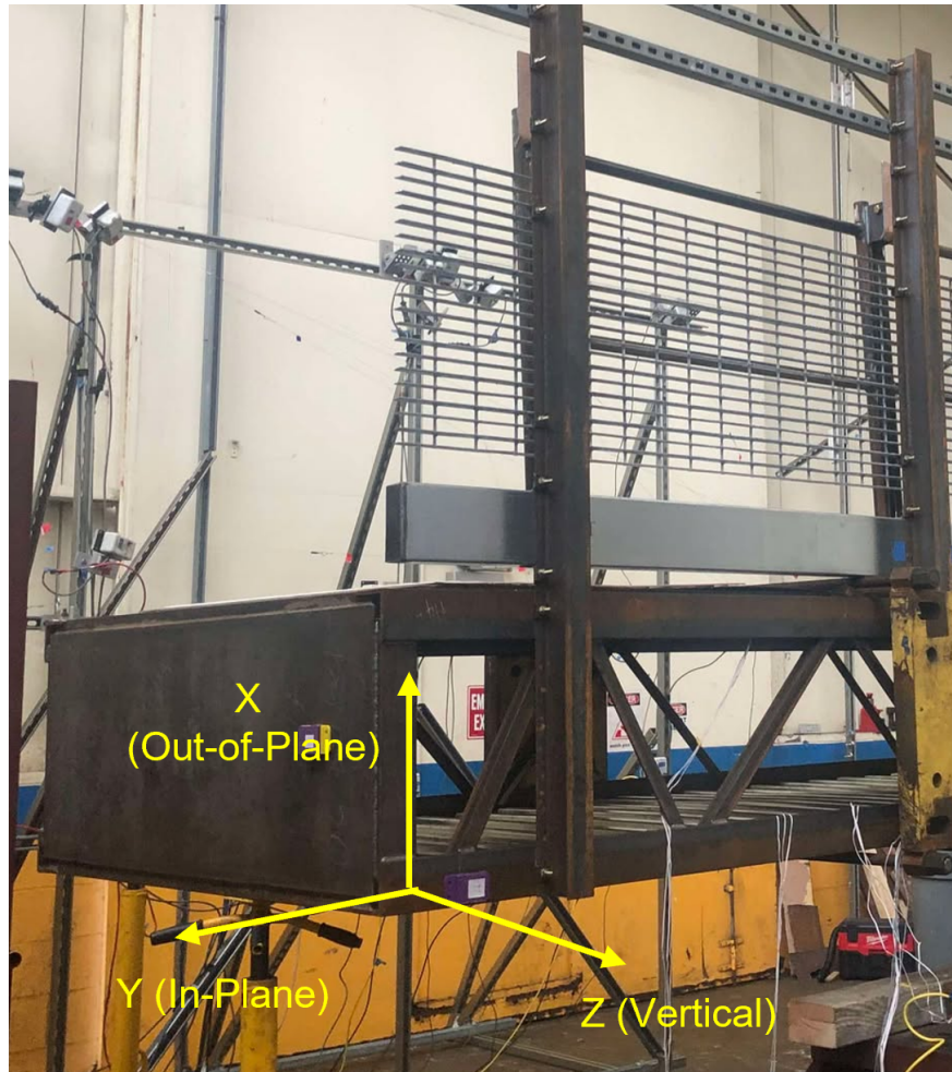
Figure 6.1: Directions used for natural period characterization and presentation of displacement results.
