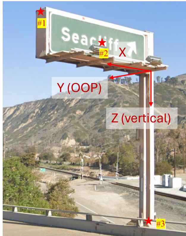
Figure 3.2: The locations of PEER-CENTS used in the field tests.
