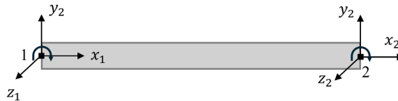
Figure 2.3: 1D beam elements
