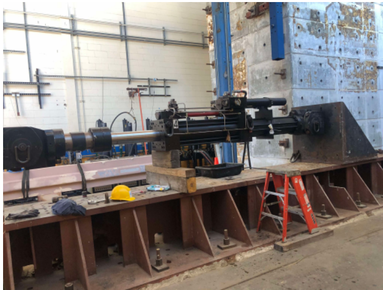
Figure 5.4: The actuator in PEER lab
