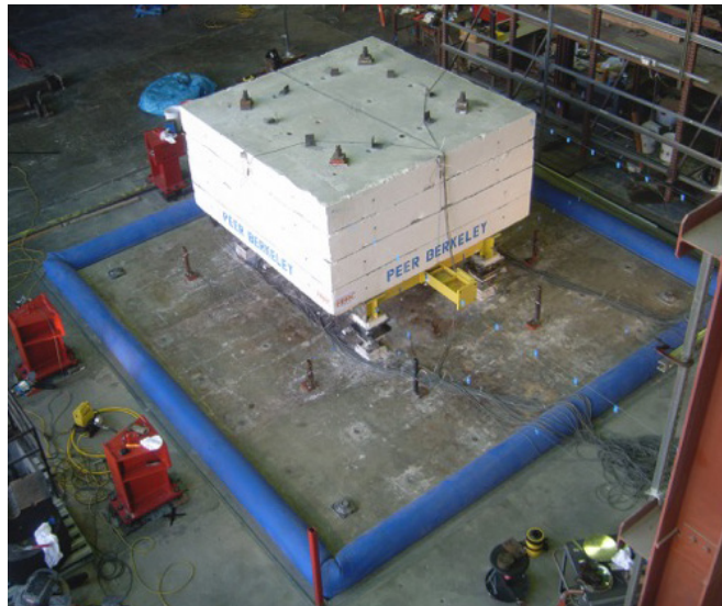
Hybrid Testing of Tuned Mass Damper System
