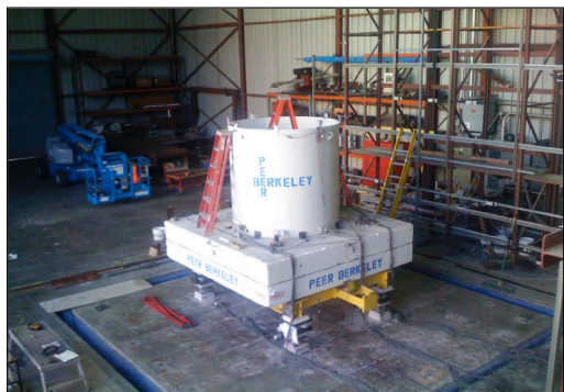
Liquid Storage Tank & Isolation System
