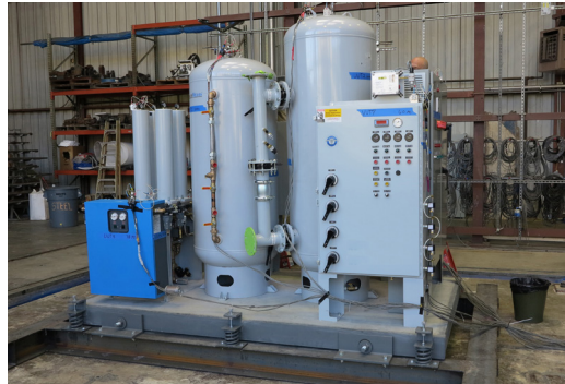
Equipment Testing (AC-156)
