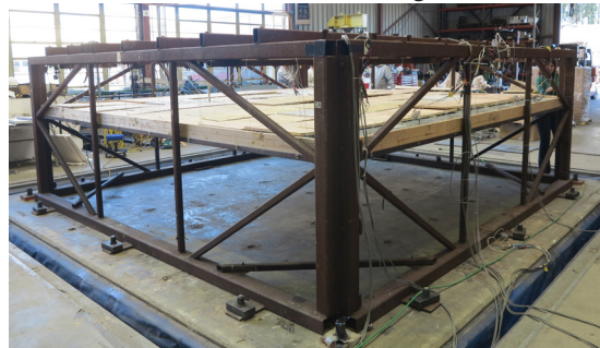
Ceiling Assembly Testing
