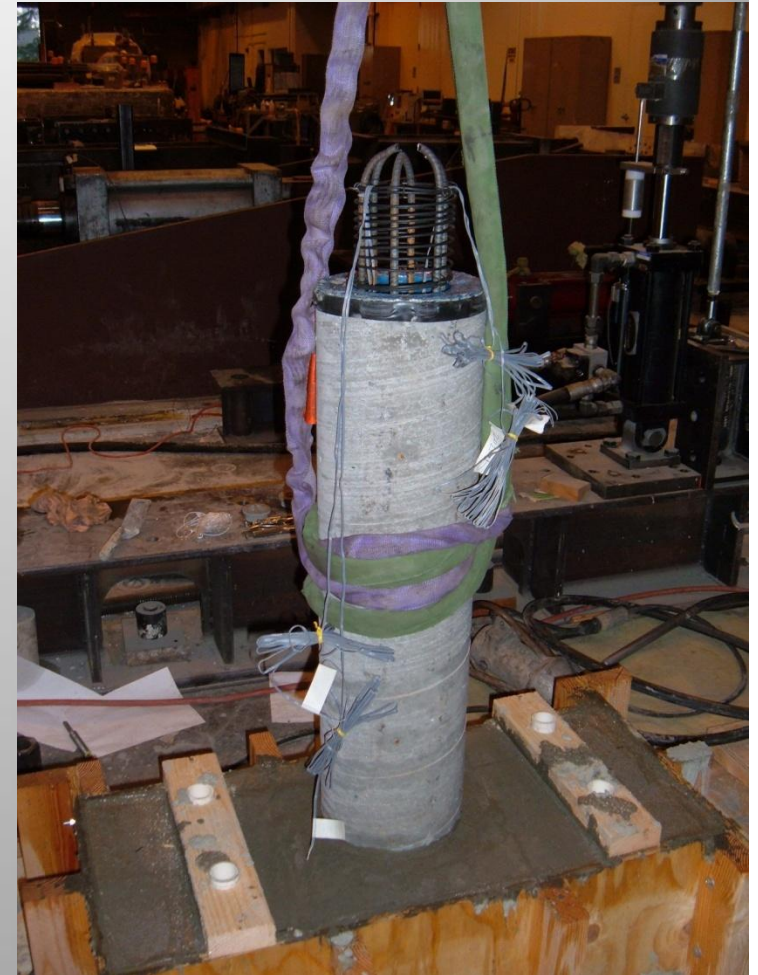
Sliding of SC-HyFRC tube over pre-existing longitudinal reinforcing cage (shown here for small scale specimen)
