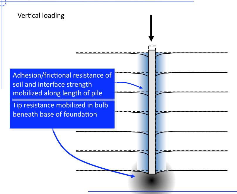
Analysis of deep foundation response – vertical loading, single foundation
