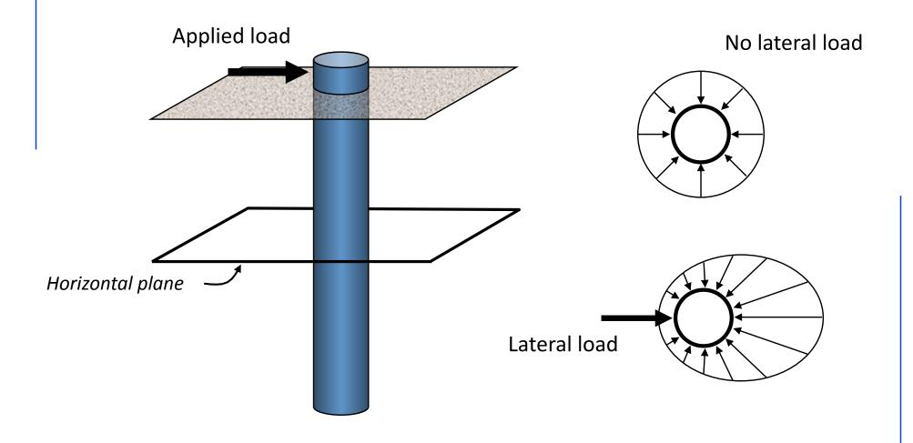
Single pile/shaft behavior – lateral loading
