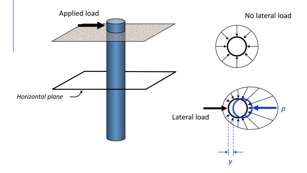
Single pile/shaft behavior – lateral loading
