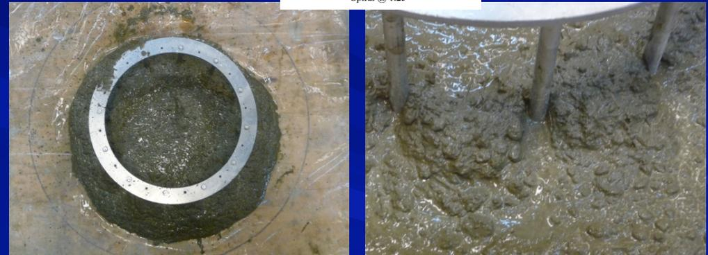
Conclusion: The volume fraction of long fibers had to be reduced to ensure sufficient flowability and homogenous fiber dispersion due to the close rebar spacing of the bridge columns
