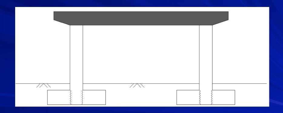
4) Set cap-beam, grout bars into ducts.
