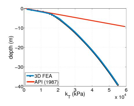
A parabolic distribution of initial stiffness, as used by Brandenberg et al. (2007) and Lam and Cheang (1995), or a similar bilinear distribution to that above is recommended for a static BNWF analysis of lateral spreading.
