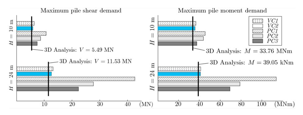
The 3D results compare well with the results obtained using p-y curves reduced using the proposed procedure for these arbitrary soil profiles
