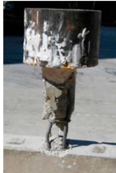
Fig. 4.43 Specimen 4 after axial crushing
