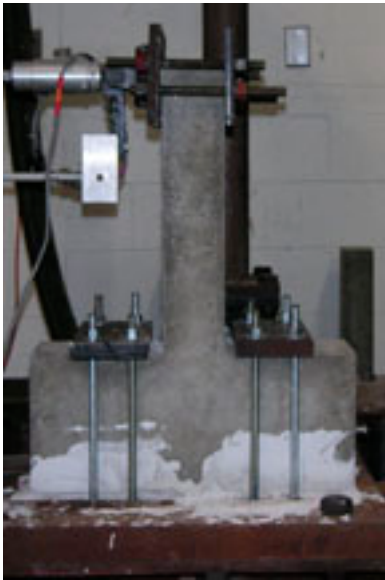
Fig. 4.42 Experimental lateral setup
