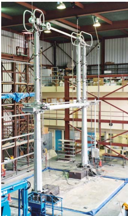
Figure 1 550-kV switch in the closed position mounted on supports
