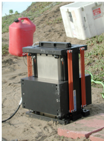
Figure 1. Electromechanical shaker in the field for swept sine wave SASW profiling.
