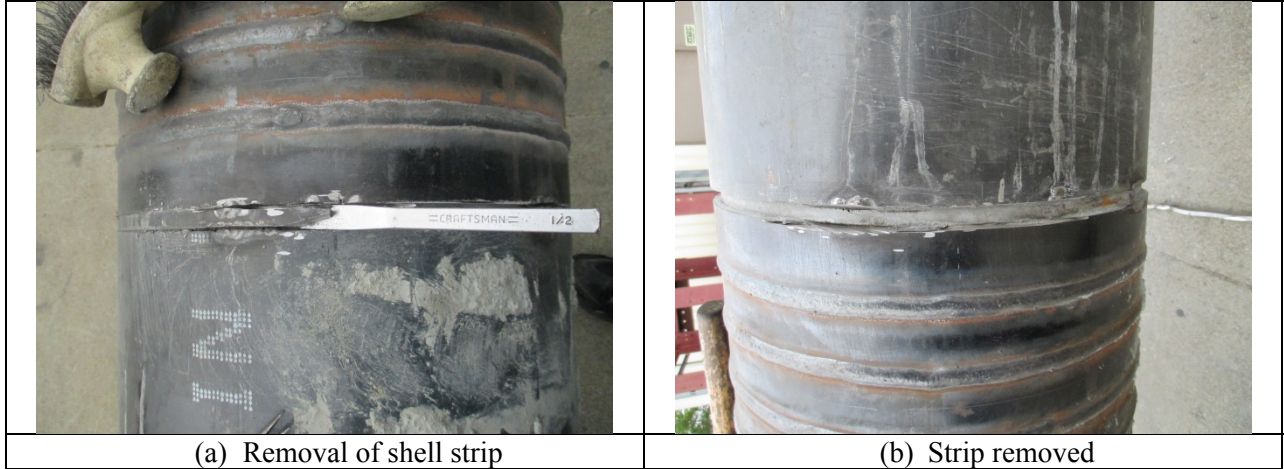
Figure 7 Specimen assembly: Preparing the rocking interface
