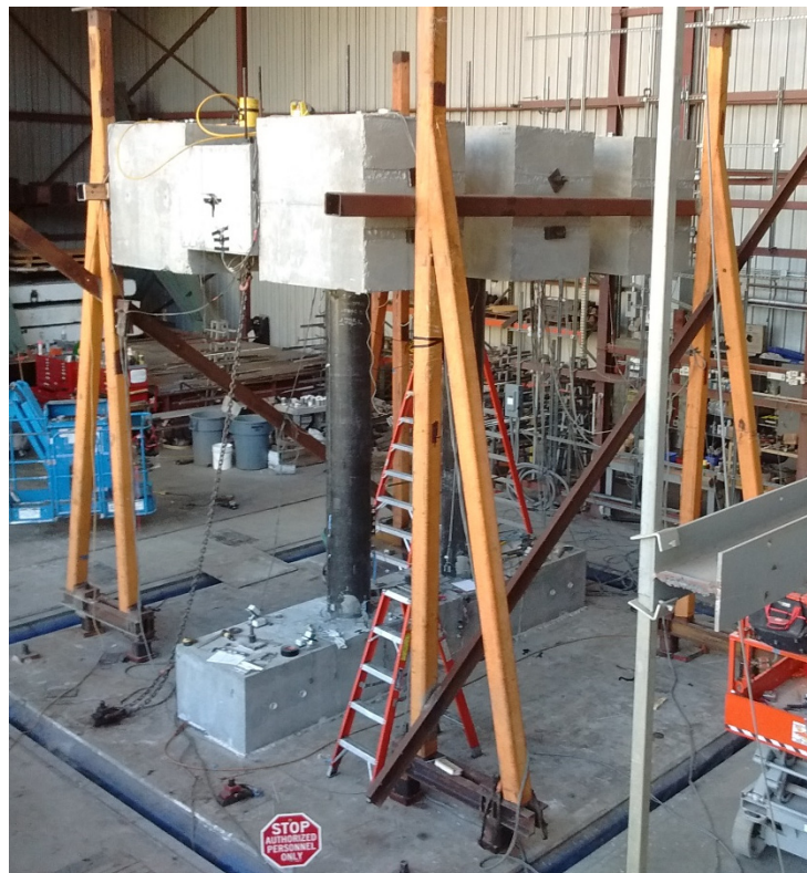
Figure 14 Completed specimen with restraint frames
