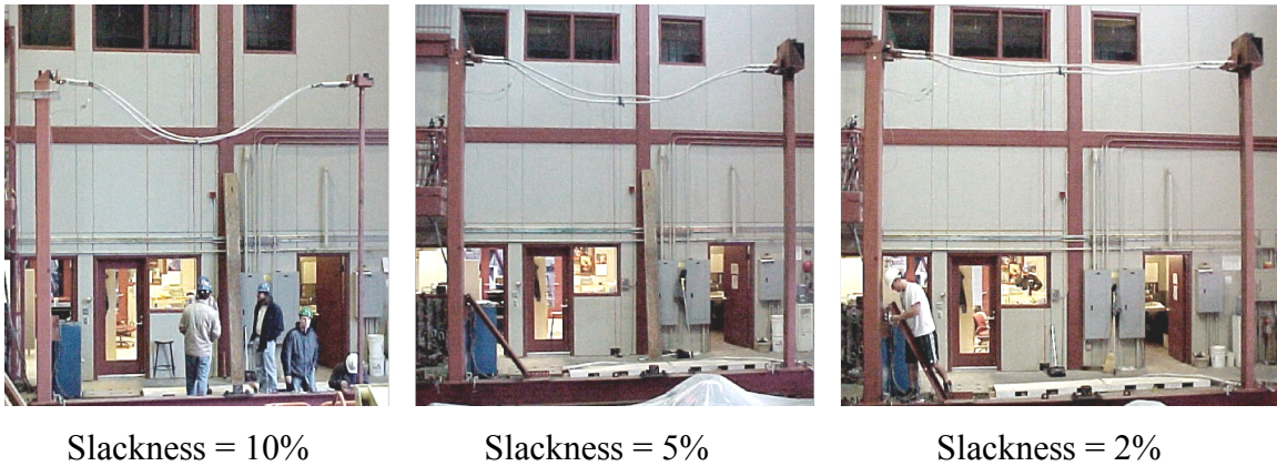
Figure 2.7 Equipment Pair 4 Connected by 1113C conductor.
