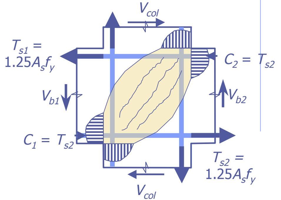
(b) internal stress resultants acting on joint
