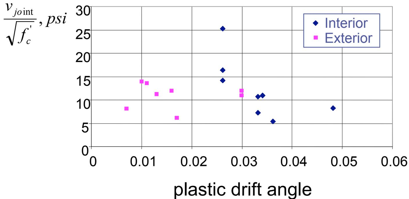
Note: the plastic drift angle includes inelastic deformations of the beams
