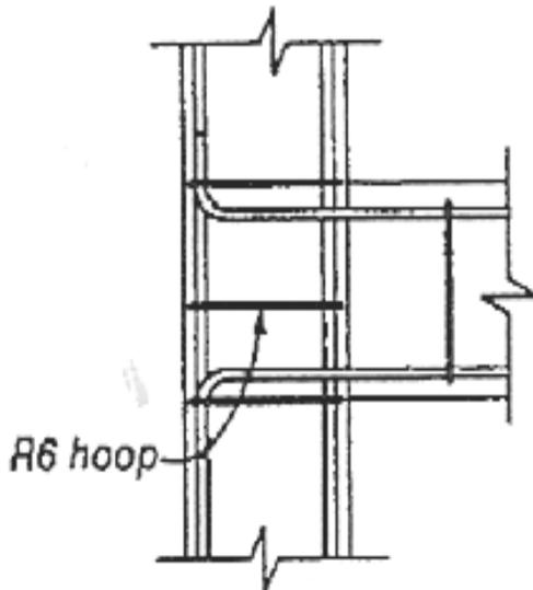
hook bent out of joint
