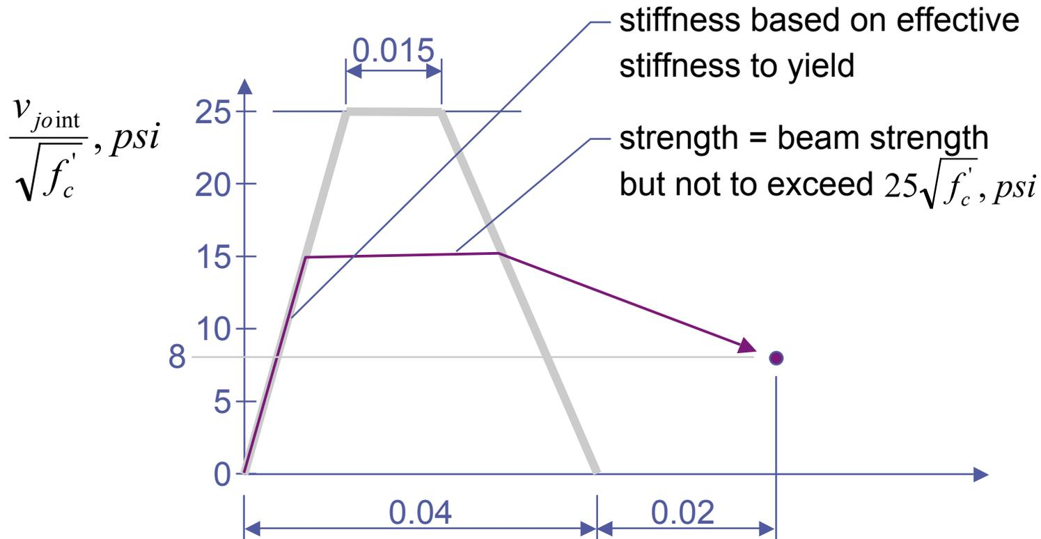
Note: the plastic drift angle includes inelastic deformations of the beams
