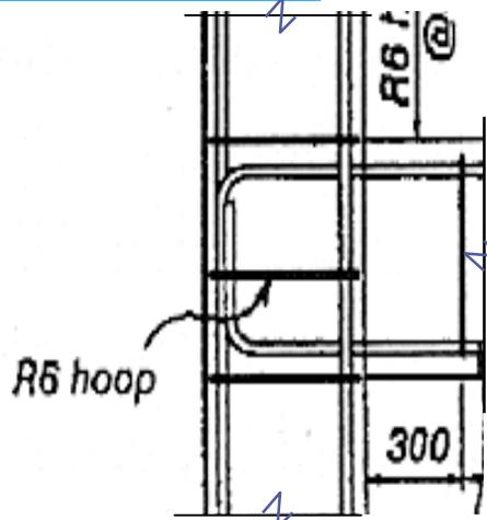
hook bent into joint
