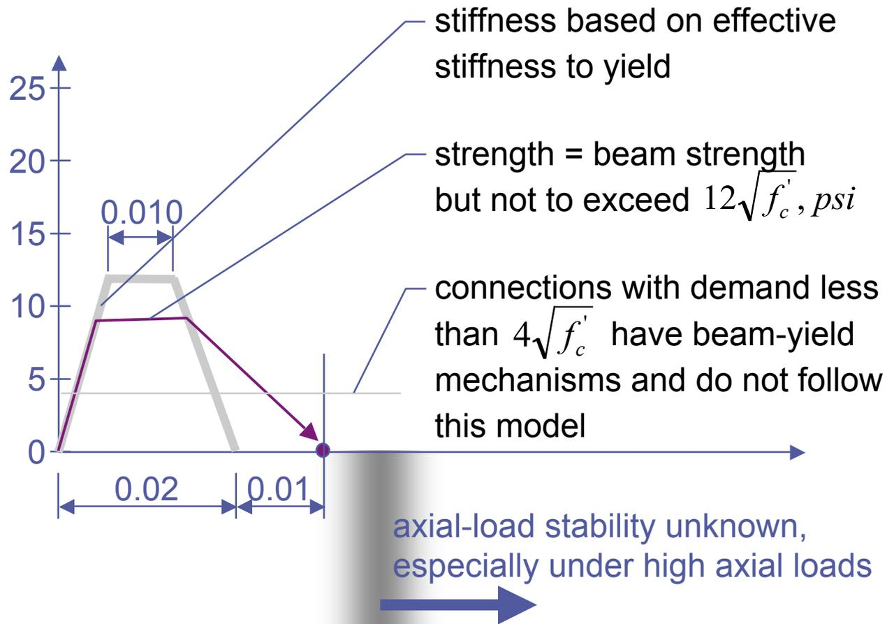
Note: the plastic drift angle includes inelastic deformations of the beams
