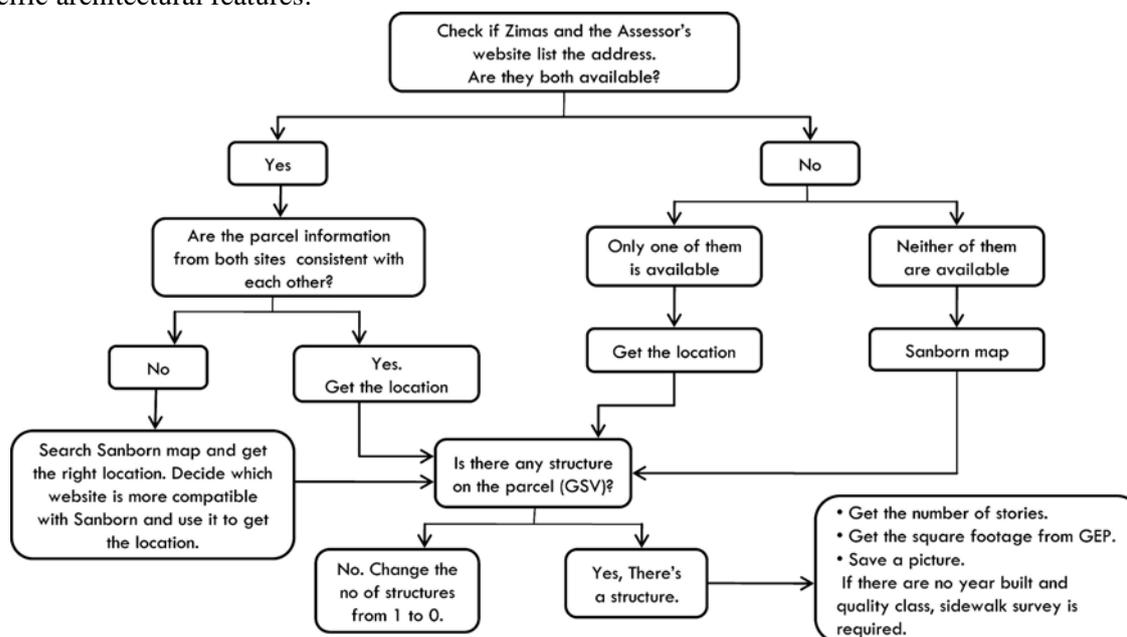
Figure 1 Flowchart of methodology for validating data
