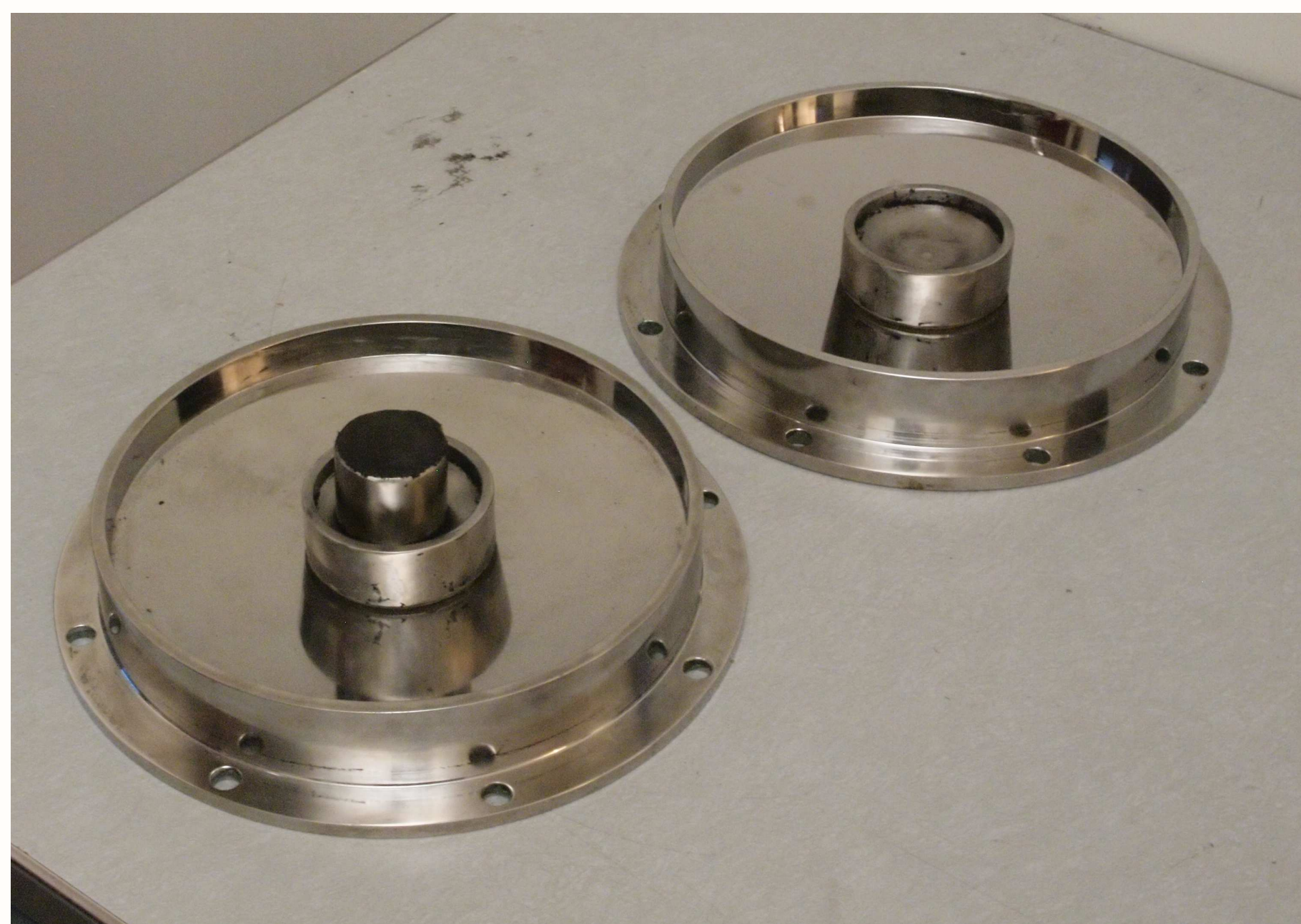
Figure: An overview image of an example of a Triple Friction Pendulum (TFP).
